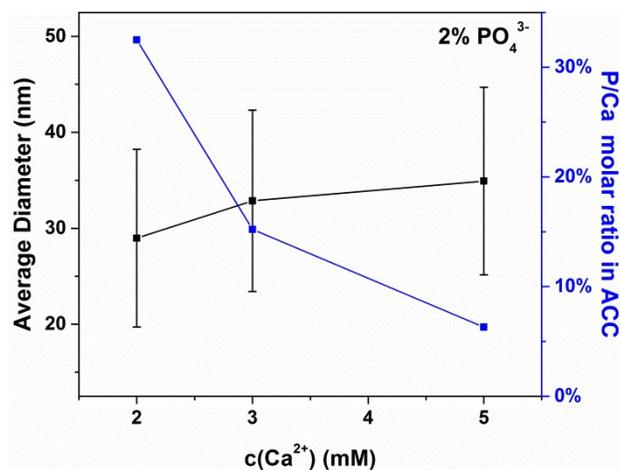
**Figure S5.** Average diameter and the P/Ca molar ratio in ACC prepared at low concentration of calcium carbonate (2 – 5 mM) in the presence of 2%  $\text{PO}_4^{3-}$ .
