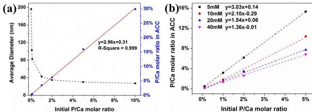
**Figure S4.** (a) The average diameter and P/Ca molar ratio in the ACC prepared at a calcium concentration of 5 mM in the presence of phosphate. (b) The P/Ca molar ratio in the ACC as a function of initial phosphate content in solution at different concentration of calcium carbonate (5 – 40 mM).
