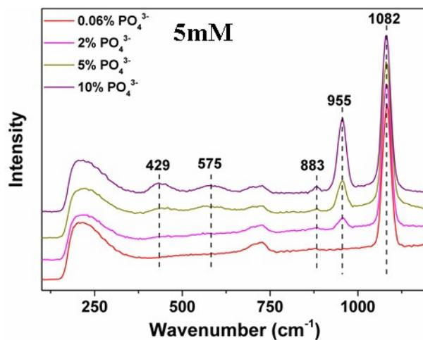
**Figure S7.** Raman spectra of ACC sample prepared in the presence of PO<sub>4</sub><sup>3-</sup> ions. The broad peak at 955 cm<sup>-1</sup> (FWHM width of ~28 cm<sup>-1</sup>) in the Raman spectra (Figure 3f) suggests that the PO<sub>4</sub><sup>3-</sup> ions in ACC existed in an amorphous state.<sup>1</sup> No sign of HPO<sub>4</sub><sup>2-</sup> was observed in these spectra.<sup>2</sup>
