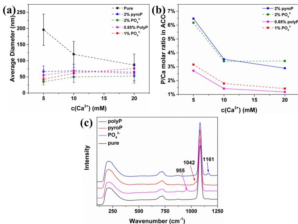
**Figure S6.** (a) Average diameter of ACC prepared at calcium carbonate concentrations of 5-20 mM in the presence of 2% (P/Ca molar ratio) of pyrophosphate (pyroP) and 0.85% of polyphosphate (P/Ca molar ratio). (b) The corresponding P/Ca molar ratio in ACC measured
