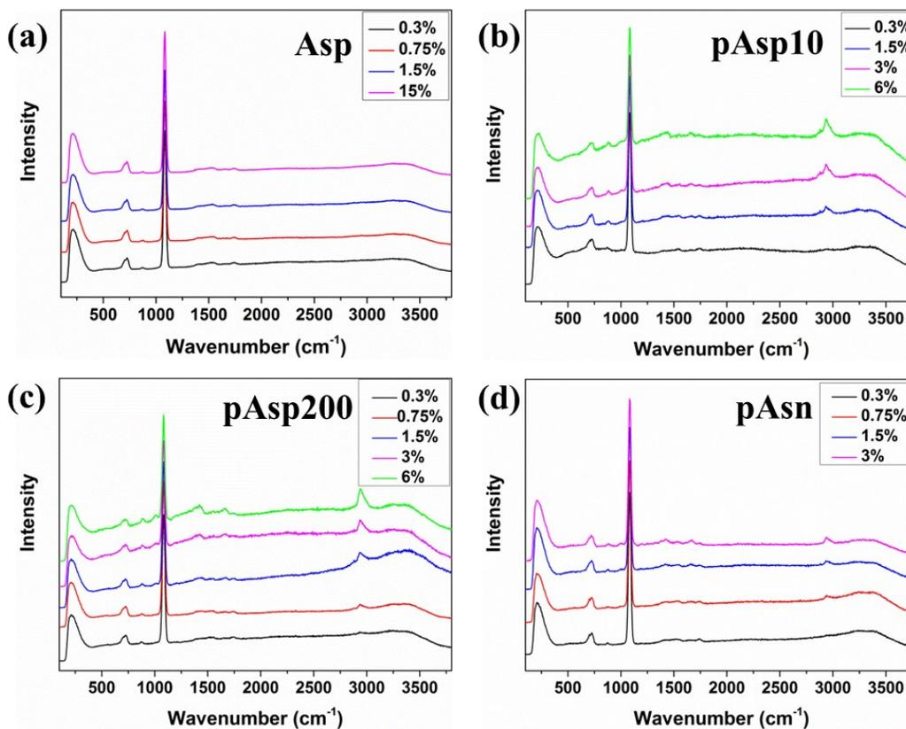
**Figure S2.** Raman spectra of ACC prepared at 5mM in the presence of different amount of Asp (a), pAsp10 (b), pAsp200 (c) and pAsn (d), showing that Asp monomer does not incorporate into ACC, while pAsp with chain length 10 and 200 and pAsn can incorporate into ACC.
