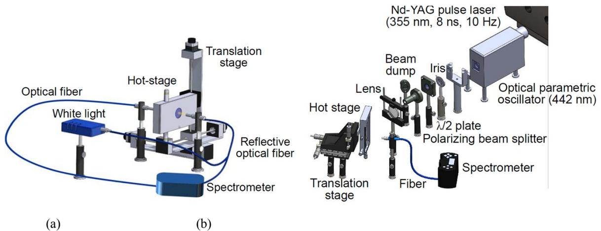
**Figure S1.** Experimental setups for measuring (a) the reflection and (b) the lasing emission spectra of the samples.
