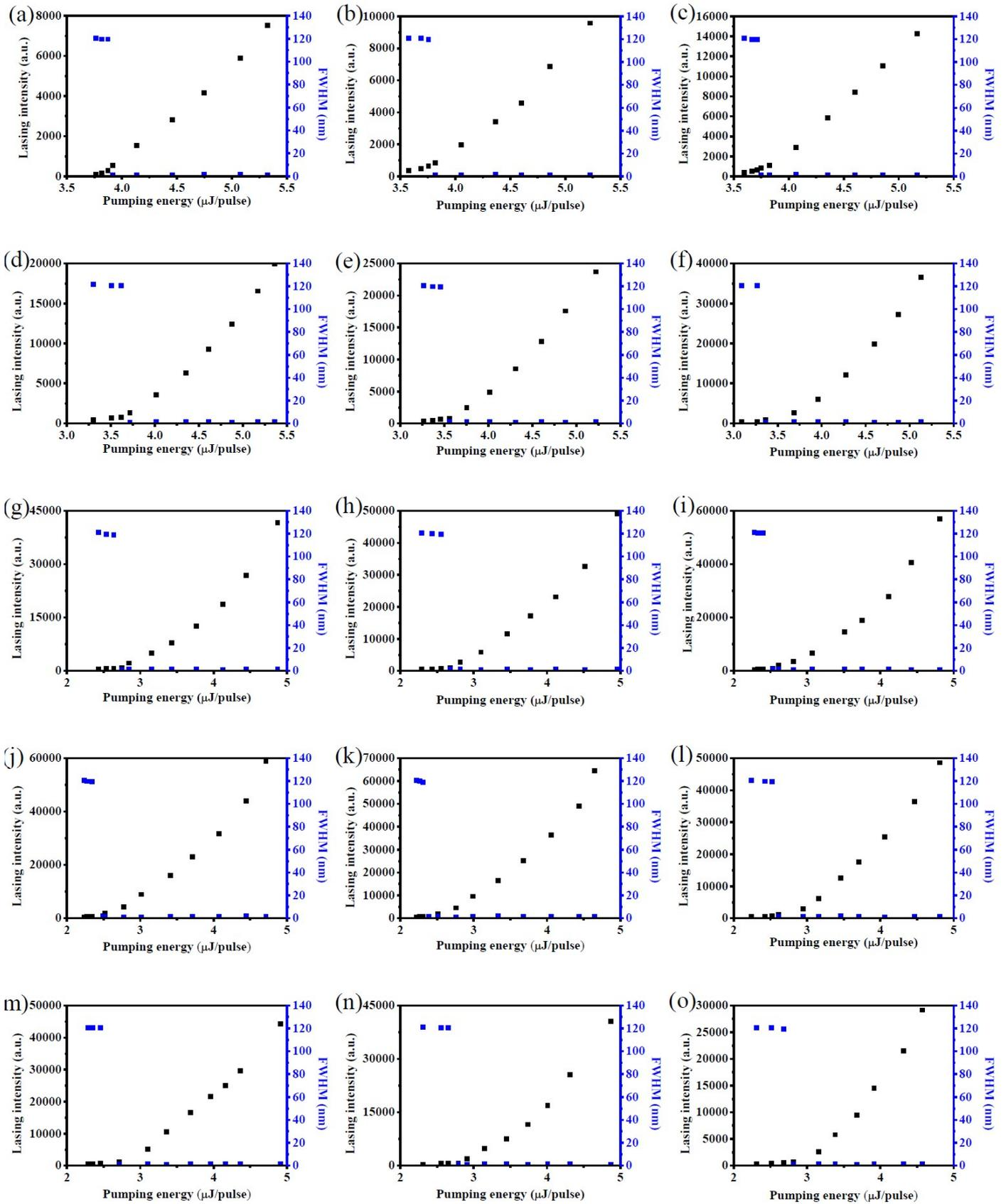
**Figure S5.** Variations of the intensity of the lasing peak and the corresponding FWHM of the lasing emission of the DDNLc-refilled gradient-pitched *enantiomorphic* template laser with pumped energy measured at positions of  $x =$  (a) 4, (b) 4.5, (c) 5, (d) 5.5, (e) 6, (f) 6.5, (g) 7, (h) 7.5, (i) 8, (j) 8.5, (k) 8.9, (l) 9.5, (m) 10, (n) 10.4, (o) 11 mm, respectively, at 48 °C.
