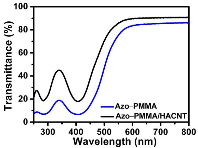
Fig. S3 UV–Vis transmittance spectra of pure Azo–PMMA and Azo–PMMA/HACNT composite film.
