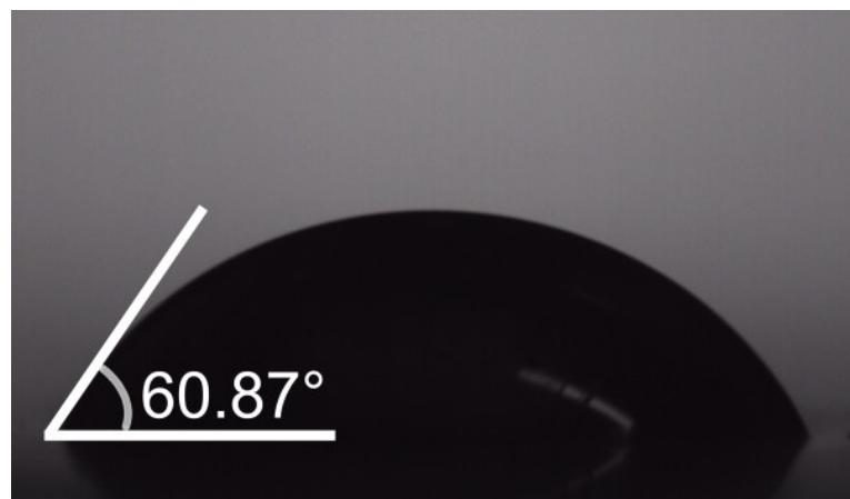
Fig. S4 Digital image of the contact angle of Azo-PMMA on unmodified HACNT film.
