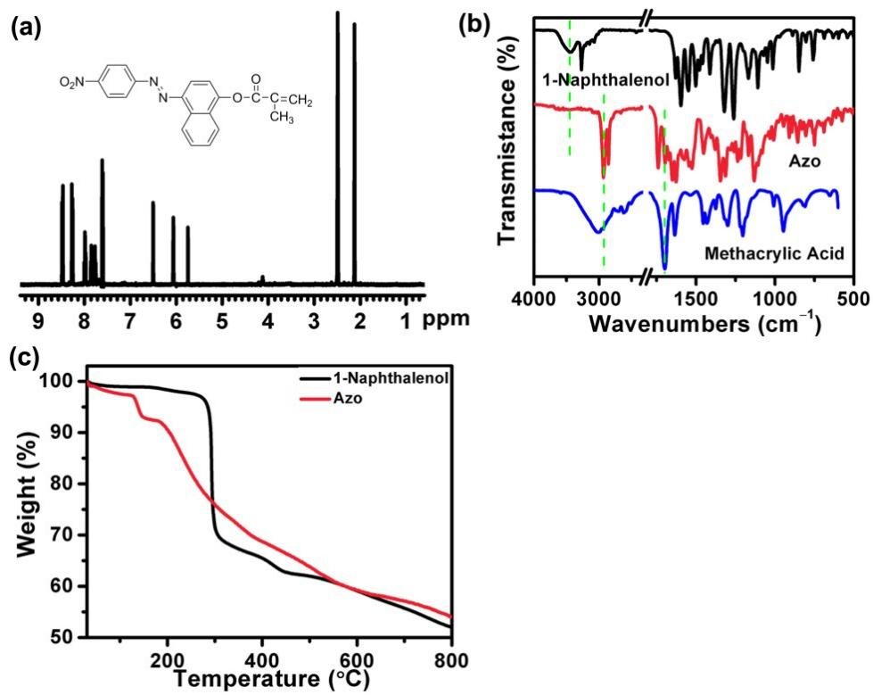
Fig. S1 Chemical structure of Azo monomers: (a)  $^1\text{H}$  NMR spectrum; (b) FTIR spectra; (c) TGA spectra.
