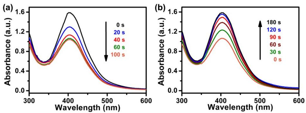
Fig. S7 UV–Vis absorption spectra changes of Azo–PMMA film: (a) upon irradiation with UV–365 nm; (b) in darkness after the irradiation.
