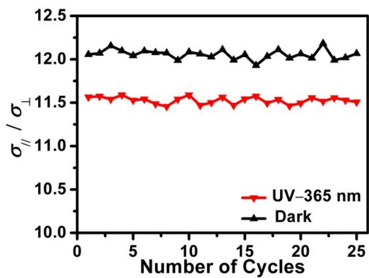
Fig. S8 Anisotropic electrical conductivity of Azo-PMMA/HACNT composite film before and after UV irradiation at 365 nm.
