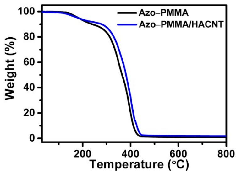
Fig. S6 TGA spectra of pure Azo-PMMA and Azo-PMMA/HACNT composite film.
