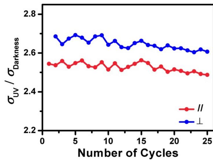
Fig. S9 Anisotropic light-induced conductance switching of Azo–PMMA/HACNT composite film.
