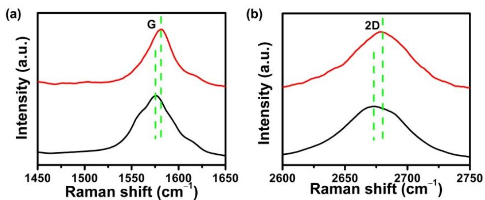
Fig. S10 Raman spectra of Azo–PMMA/HACNT composite film before and after UV irradiation at 365 nm.
