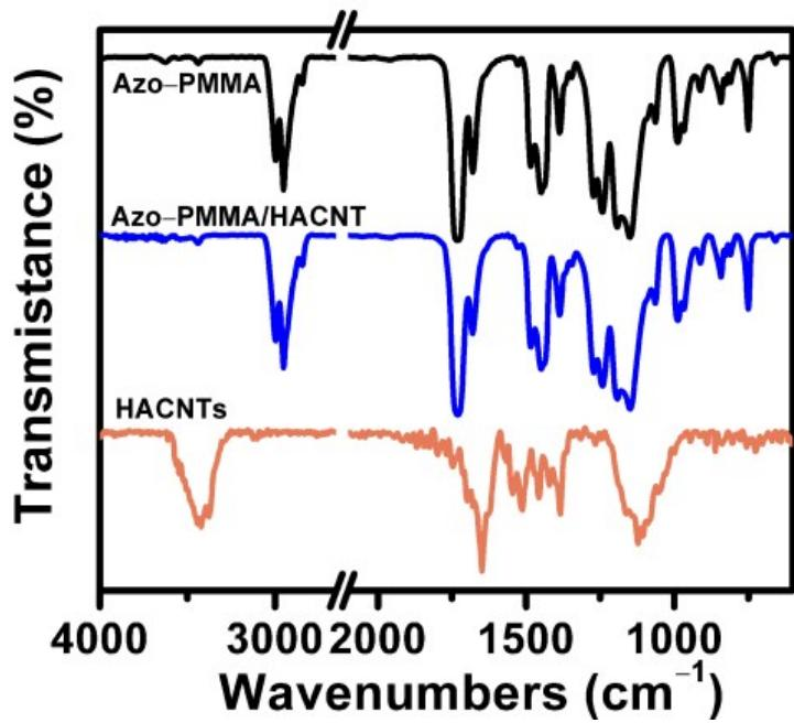
Fig. S5 FTIR spectra of HACNTs, pure Azo-PMMA and Azo-PMMA/HACNT composite film.
