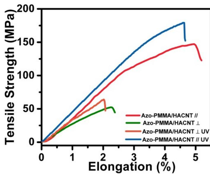
Fig. S11 Anisotropic tensile strength of Azo-PMMA/HACNT composite film before and after UV irradiation at 365 nm.
