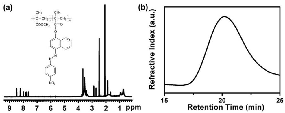
Fig. S2 Chemical structure of Azo-PMMA polymer: (a)  $^1\text{H}$  NMR spectrum; (b) GPC chromatogram.
