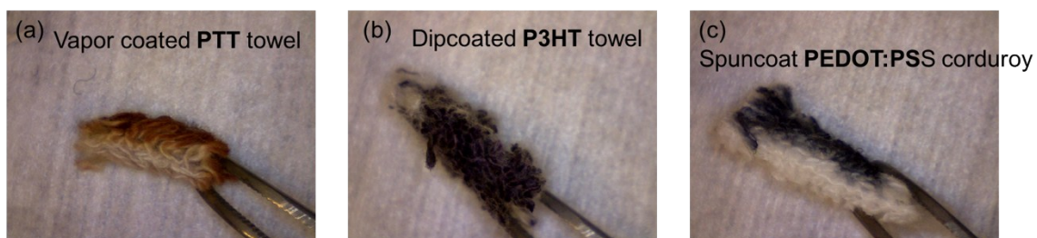
Figure S5. Photographs of the side view of (a) PTT vapor coated towel (b) P3HT dipcoated towel and (c) corduroy spun coat with PEDOT:PSS. Dipcoating fully dyes the towel but vapor deposition and spincoating result in primarily surface coatings.
