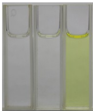
Figure S-4. Photo of 1 \times 10^{-5} M PTZ, TAC and TPTZ-TAC1 in benzene: MeCN ( v:v=1:1 ) from left to right.
