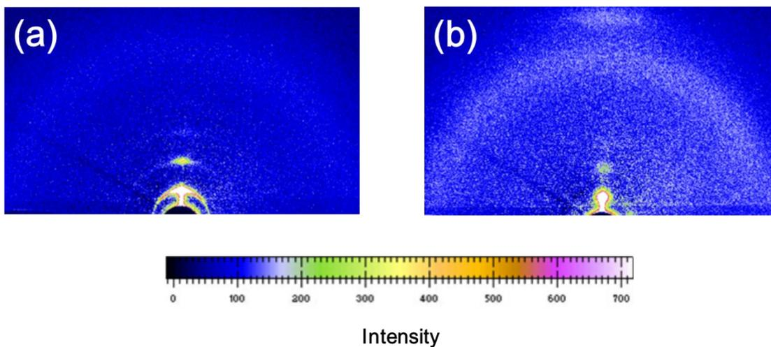
**Figure S5.** Grazing incidence wide-angle X-ray diffraction (GIXD) patterns of (a) FBT-DTh<sub>DT</sub>-TT-L film and (b) FBT-DTh<sub>DT</sub>-TT-H film.
