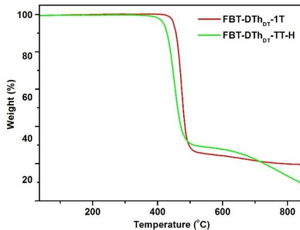
**Figure S1.** Thermogravimetric analysis of FBT-DTh<sub>DT</sub>-1T and FBT-DTh<sub>DT</sub>-TT-H at a heating rate of 20 °C/min under a nitrogen atmosphere.
