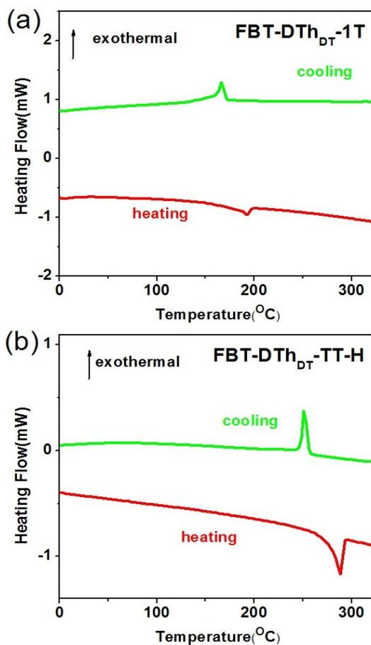
**Figure S2.** Differential scanning calorimetry thermograms of FBT-DTh<sub>DT</sub>-1T (a) and FBT-DTh<sub>DT</sub>-TT-H (b) at a heating or cooling rate of 10 °C/min under a nitrogen atmosphere.
