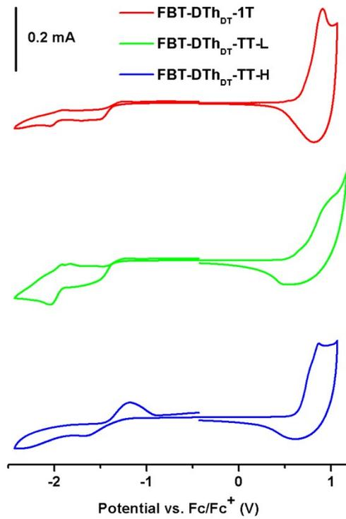
**Figure S3.** Cyclic voltammogram of polymers with an Ag/Ag<sup>+</sup> electrode as the reference electrode and an energy level of ferrocene of -4.80 eV as the internal standard.
