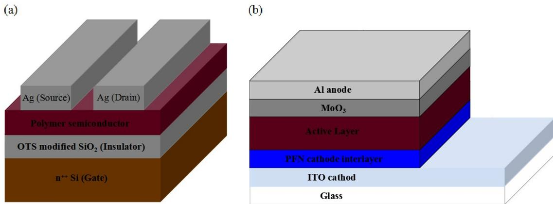
**Figure S4.** Device configurations of (a) the top-contact field effect transistors and (b) the inverted polymer solar cells.
