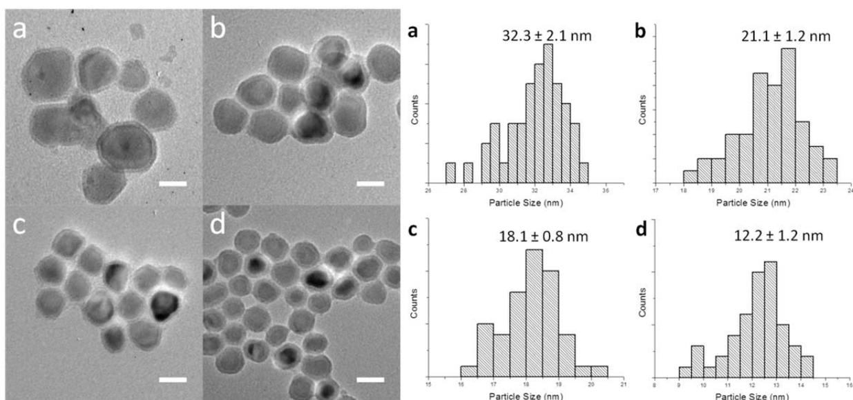
**Fig. S1.** TEM images and size distribution histograms of synthesized MnAs nanoparticles prepared according to a published procedure<sup>1</sup> (1 mmol Mn and As atomic concentrations, 5 g of TOPO and 10 mL of octadecene) but varying the reaction time: (a) 10 h (b) 5 h (c) 2 h (d) 1 h (the scale bar is 20 nm).
