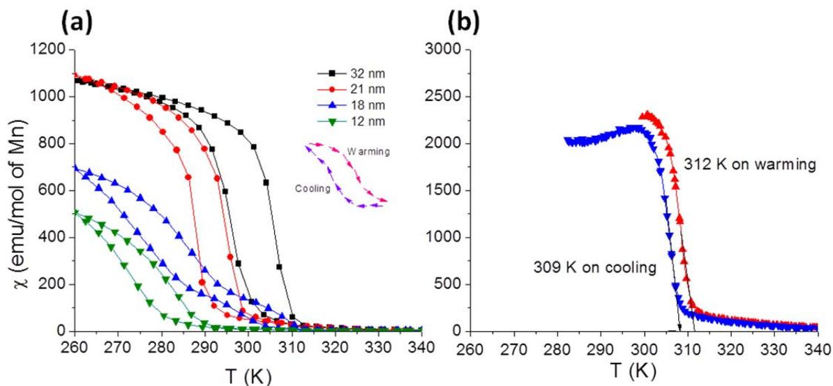
**Fig. S3.** Comparison of the temperature dependent magnetic susceptibility (magnetic susceptibility per mole of Mn) for (a) type-B MnAs nanocrystals (from 12 to 32 nm) and (b) type-A MnAs nanoparticles (22 nm). The temperature dependent magnetic susceptibility of 21 nm type-B MnAs nanocrystals adopting the  $\beta$  structure was previously reported.<sup>1</sup> The presence of two transitions in the 18 nm samples may reflect a small degree of type-A impurity (with a higher  $T_C$ ).
