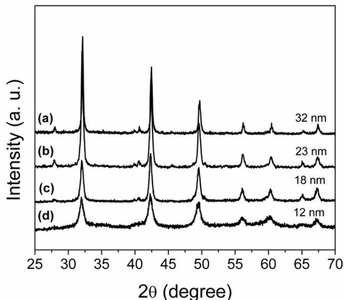
**Fig. S2.** The XRD patterns of synthesized MnAs nanocrystals prepared according to published methods<sup>1</sup> (1 mmol Mn and As atomic concentrations, 5 g of TOPO and 10 mL of octadecene) but varying the reaction time: (a) 10 h (b) 5 h (c) 2 h (d) 1 h. The drop lines indicate the reference spectrum of the  $\beta$ -MnAs (PDF# 71-0923). The crystallite size achieved by application of the Scherrer equation is indicated.
