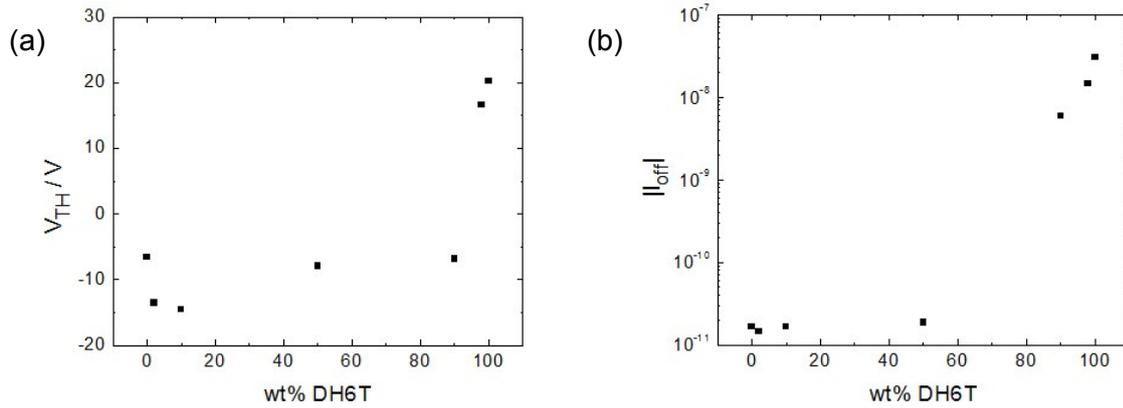
**Fig. S5.** Threshold voltages (a) and off currents (b) as a function of the amount of DH6T added to DH4T. All the transfer curves are recorded in devices with with  $L = 10 \mu\text{m}$  and  $W = 10 \text{mm}$ .
