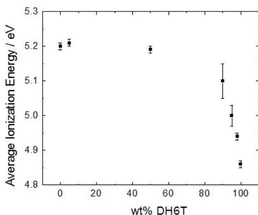
**Fig. S8.** Ionization energy as a function of the amount of DH6T added to DH4T.
