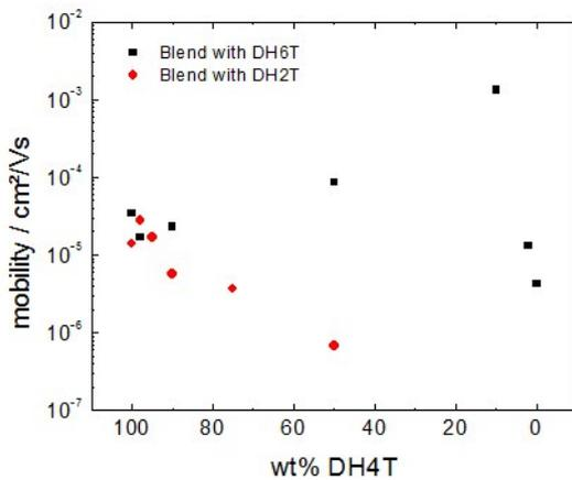
**Fig. S6.** Mobility as a function of DH4T wt% in a blend with either DH6T or DH2T. Field-effect mobility values were obtained from transfer curves (average over 8 transistors with  $L = 2.5 \mu\text{m}$ ;  $5 \mu\text{m}$ ;  $10 \mu\text{m}$ ;  $20 \mu\text{m}$ ).
