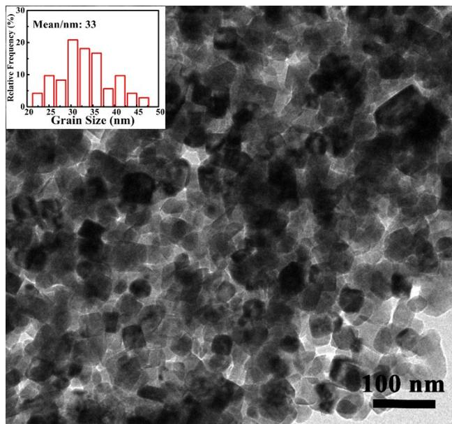
Fig. S1. TEM micrograph of pure KNN powder and the inset shows the grain size distribution.
