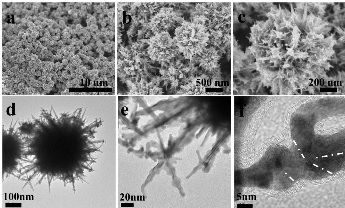
Figure S4. SEM and TEM images at different magnifications of supra-structure of AuMFs containing of hyper-branched tips synthesized by adding 120  $\mu\text{L}$  NaCl (1.0) into the growth solution from a NaCl stock solution (1.0 M). The white dash-lines indicate the twin planes.
