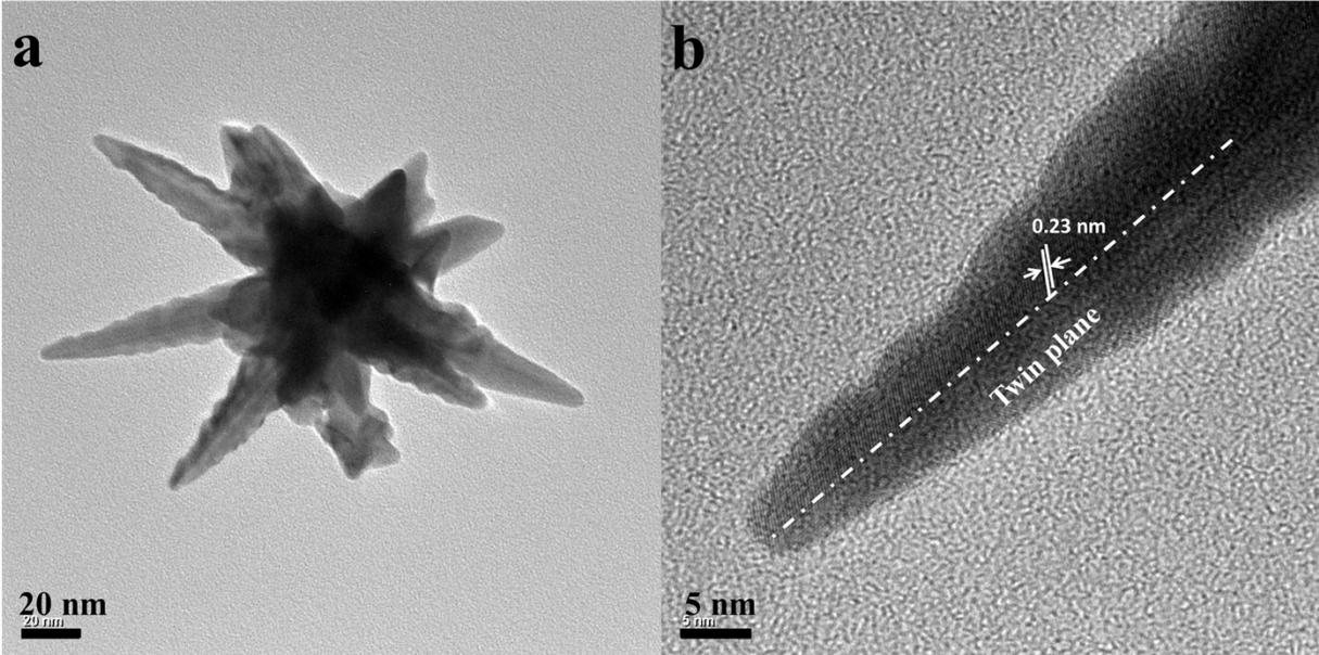
Figure S2. (a) TEM image of gold nanostars in Figure 2a synthesized upon replacing 30  $\mu\text{L}$  of HCl (1.0 M) by 15  $\mu\text{L}$   $\text{H}_2\text{SO}_4$  (1.0 M) and (b) HRTEM image of a single tip.
