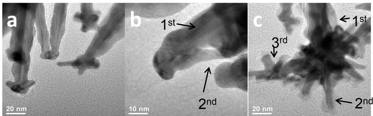
Figure S3. Additional TEM images of multilevel tips with different branching levels corresponding to branched AuMFs shown in Figure 3c and 3f, respectively: (a) tip heads, (b) 2<sup>nd</sup> tip and (c) 3<sup>rd</sup> tip.
