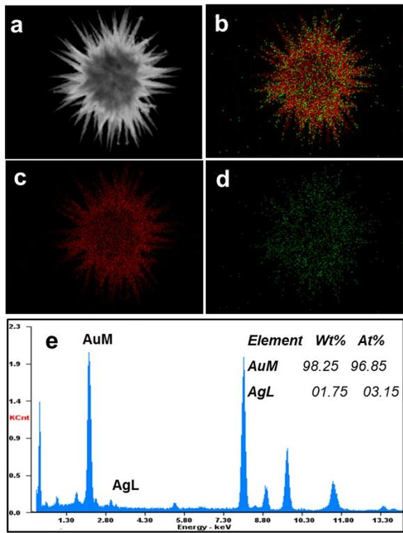
Figure S1. (a) STEM image, (b) over lapping elements, (c) gold element, (d) silver element, and (e) EDX–spectrum of branched AuMFs synthesized at typical condition: 30  $\mu\text{L}$  HCl (1.0 M), 180  $\mu\text{L}$  HAuCl<sub>4</sub> (10 mM), 20  $\mu\text{L}$  AgNO<sub>3</sub> (10 mM), and 150  $\mu\text{L}$  ascorbic acid (10 mg/mL).
