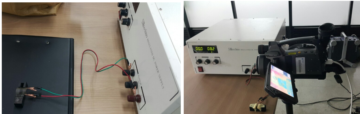
Fig.S6. Digital photograph of an experimental set up (infrared thermal imaging camera) for temperature measurement of E-PVA@Ag NF network TCE heater.
