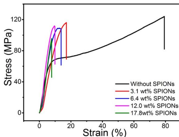
**Fig. S3** Stress-strain curves of PPy films with or without SPIONs. The number indicates the weight percentage of SPIONs in the PPy films.
