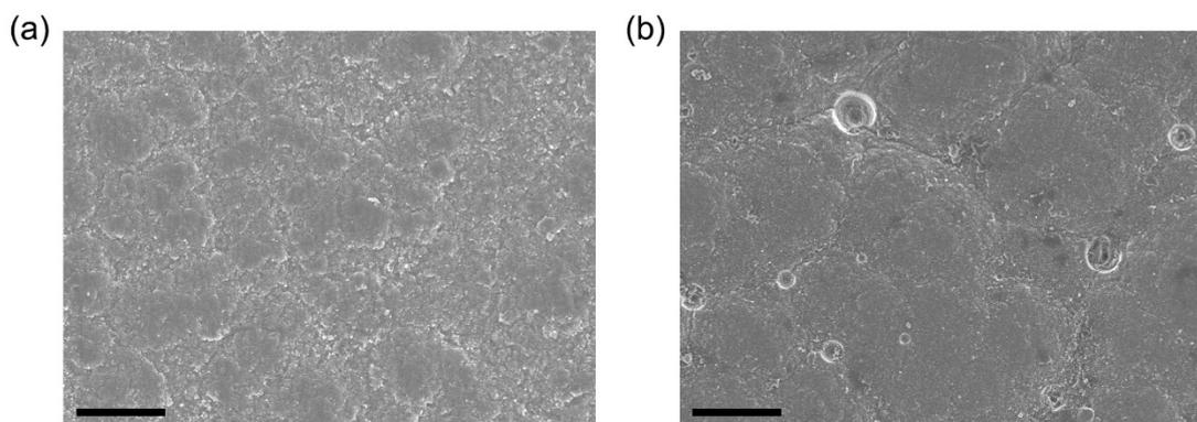
**Fig. S2** SEM images of a PPy film without SPIONs (a) and a SPIONs-PPy film (b). Scale
