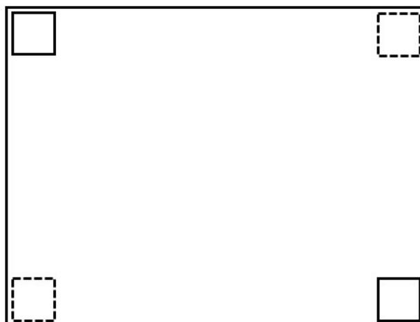
**Fig. S4** Pattern of copper sheets attachment to corners of the SPIONs-PPy film. The film is expressed as the rectangular block. Four attached copper sheets are illustrated as small square: two (solid lines) are placed on the top face of the film and the other two (dashed lines) are on the bottom face.
