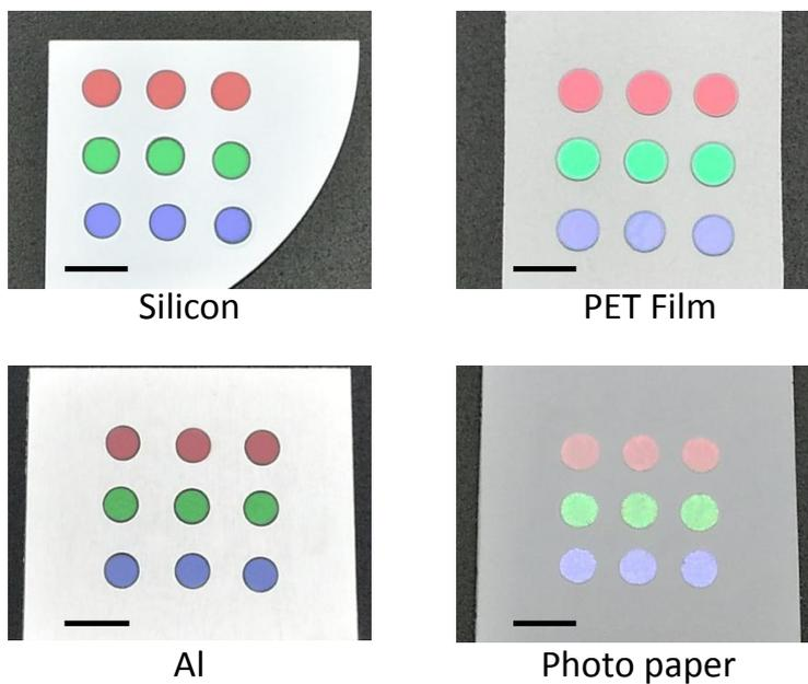
**Figure S2 Photos of prepared PCP on other different substrate:** silicon, polyethylene glycol terephthalate (PET) film, aluminum sheet and photo paper. The scale bar, 5 mm.
