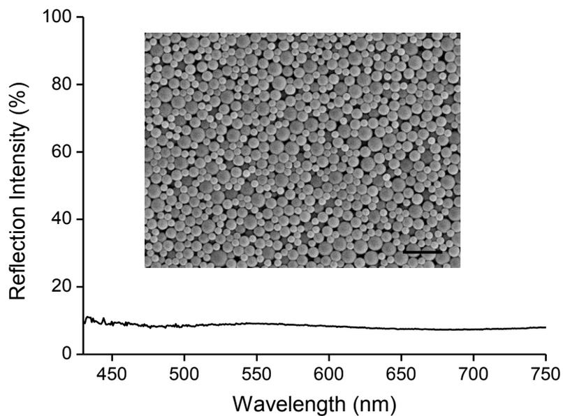
**Figure S4 Broadband reflection spectrum of the white dot prepared by the deposition of polydispersed PS particles.** Inset SEM image shows the amorphous arrangement of the polydispersed nanoparticles. The scale bar of the inset SEM image, 1  $\mu\text{m}$ .
