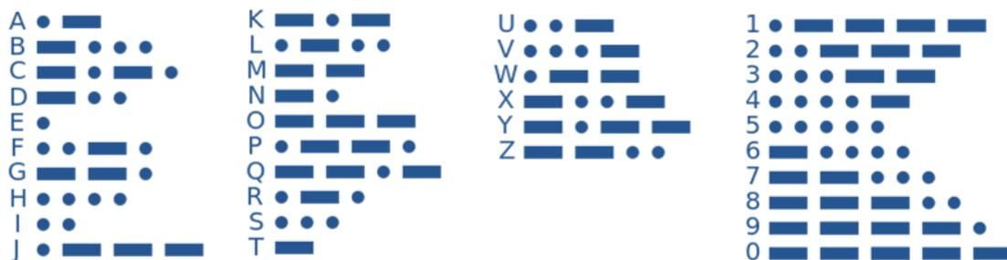
**Figure S6 The rule of International Morse Code.** The letters and numbers are marked as the modified rules above.
