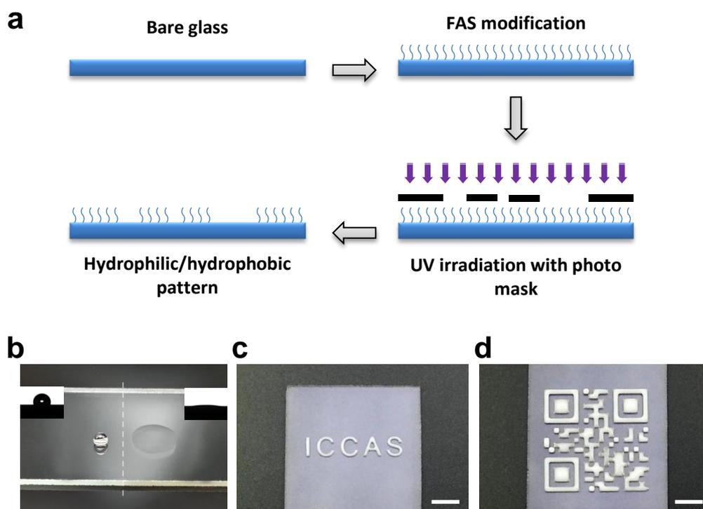
**Figure S3** The preparation process of the substrate with patterned wettability by photolithography method. **a**, Scheme of the patterning process. **b**, Contact angle of the hydrophobic ( $CA=108.5 \pm 3.5^\circ$ ) and the hydrophilic ( $CA=2.7 \pm 2.5^\circ$ ) area respectively. **c**, **d**, Photos of the patterned emulsion on the wetting patterned substrate before drying. The scale bar, 5 mm in **c** and **d**.
