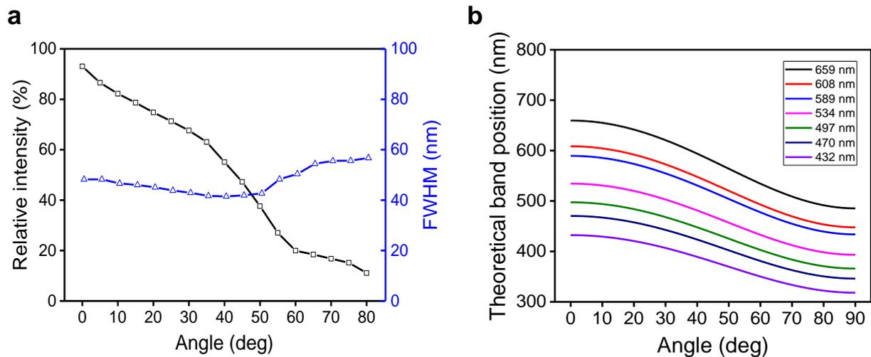
**Figure S7 Angle dependent property of photonic crystal. a,** Reflection intensity and full width at half maximum (FWHM) in different angle of the red PC dot. **b,** Theoretical angle dependent stopband of the seven typical structure colors.
