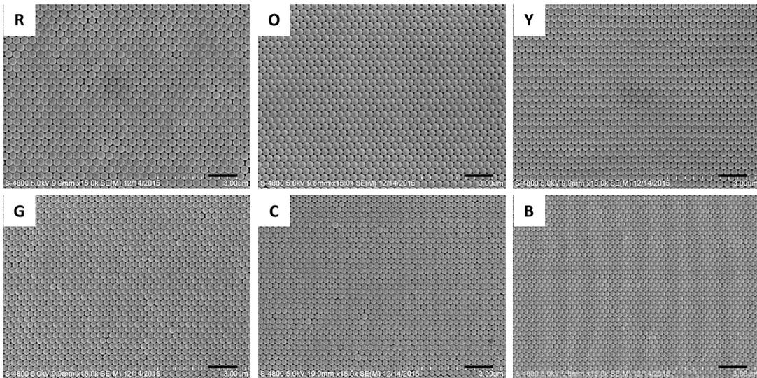
**Figure S1 SEM images of ordered nanoparticle assembly in different color PC dots:** Red-R, Orange-O, Yellow-Y, Green-G, Cyan-C, Blue-B. The color variation originates from the periodic
