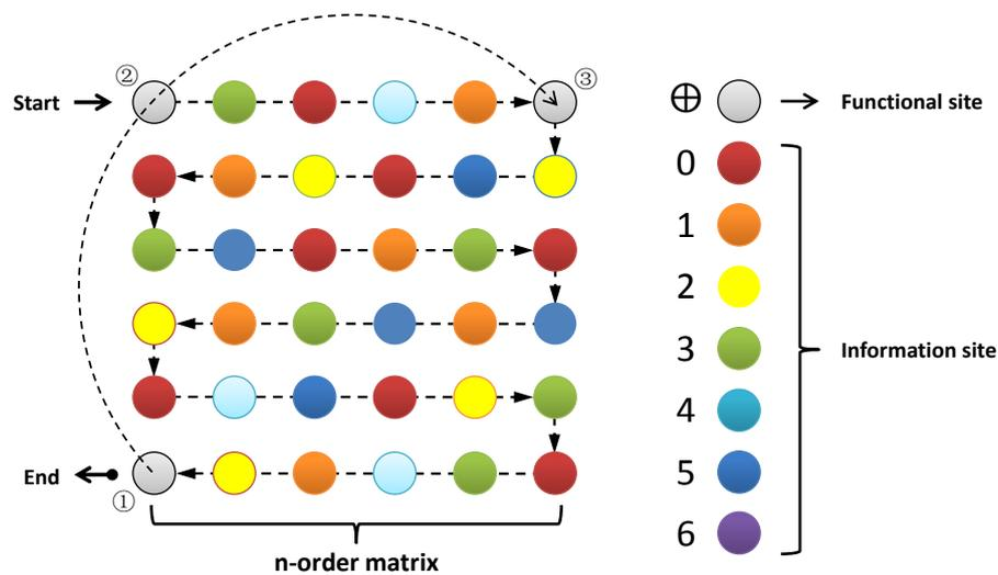
**Figure S5 Demonstration of the functional sites in the coding pattern.** The white dot of broadband reflection (marked as  $\oplus$ ) is designed as the functional site for recognition, localization, start/termination signal; the color dot (marked as 0~6) are designed as the information sites. This one white dot and the seven color dots constitute the septenary coding system.
