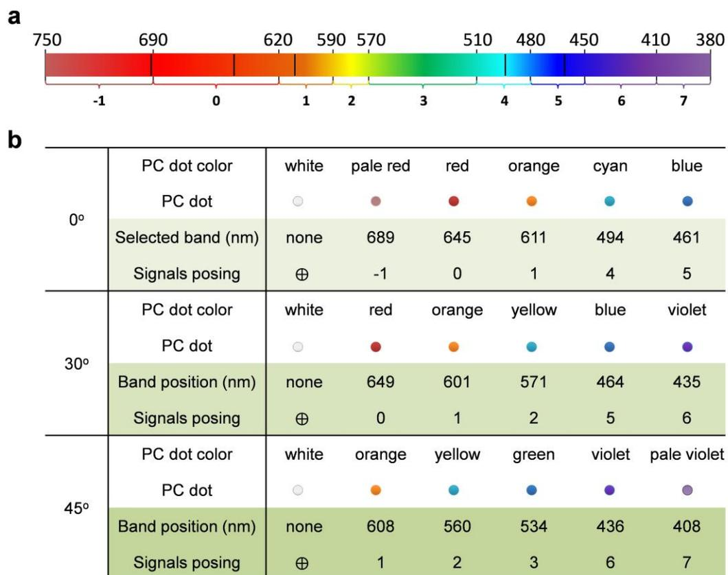
**Figure S8 Selected optical stopband for angle encryption.** **a**, A rescaled coding table for angle encryption by dividing the visible spectrum into eight parts and marked with numbers. **b**, Table of the selected stopband and corresponding digital signal. Blue shift of the stopband induces signal displacement for angle encryption.
