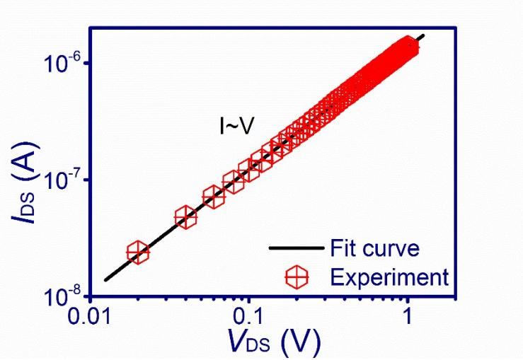
**Fig. S3**  $I_{DS}$ - $V_{DS}$  curves of the CdS-CdMoO<sub>4</sub> core-shell NR plotted in double logarithmic scales. The curves were fitted with straight lines according to the relation of  $I_{DS} \sim V_{DS}$ .
