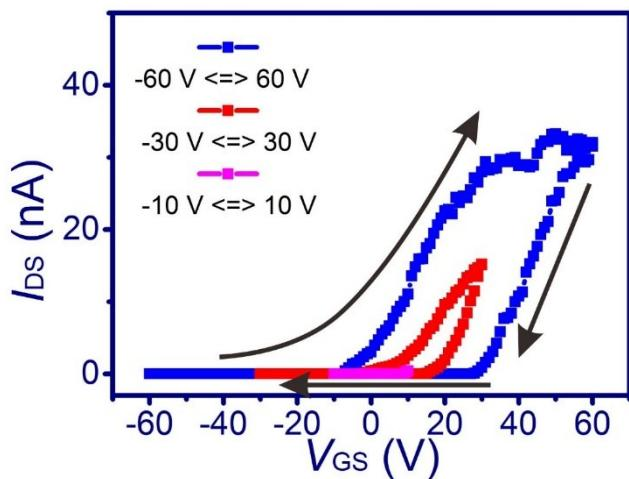
**Fig. S2** Electrical transfer characteristics of intrinsic CdS NR based NVM devices at different operating voltages with linear coordinate.
