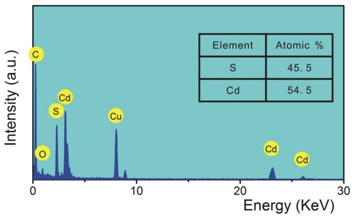
**Fig. S1** EDS spectrum of the CdS-CdMoO<sub>4</sub> core-shell NRs.
