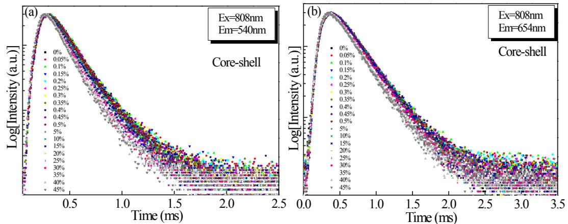
Figure S12 Water-content-dependent UC emission decay curves of (a)  $\text{Er}^{3+}$ :  $^2\text{H}_{11/2}$ ,  $^4\text{S}_{3/2}$  emitting states ( $\lambda_{\text{em}} = 540$  nm) and (b)  $^4\text{F}_{9/2}$  one ( $\lambda_{\text{em}} = 654$  nm) for the core-shell NCs under the excitation of 808 nm laser.
