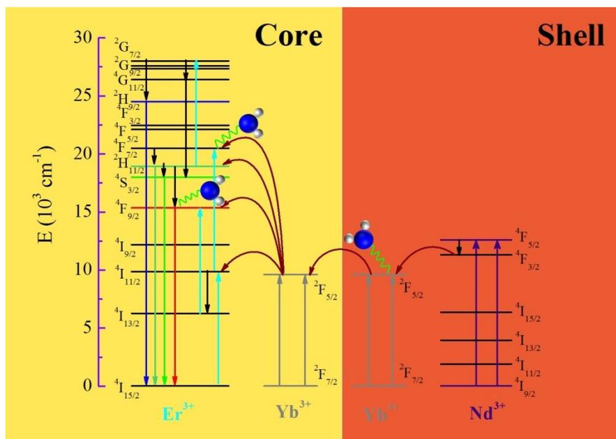
Figure S3 Energy level diagrams of Er<sup>3+</sup>, Yb<sup>3+</sup> and Nd<sup>3+</sup> ions, Nd<sup>3+</sup>-sensitized UC processes as well as the proposed mechanisms for water detection under 980nm or 808 nm excitation for the present UCNCs.
