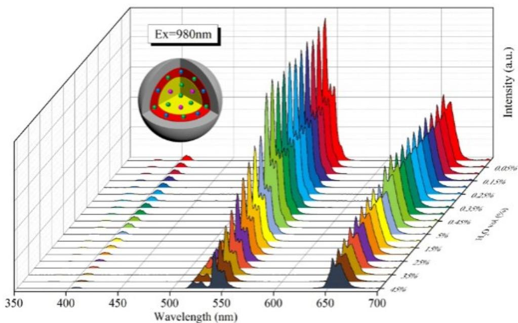
Figure S7 UC emission spectra of core-shell-shell UCNCs dispersed in DMF solution with different water contents under the excitation of 980 nm laser.
