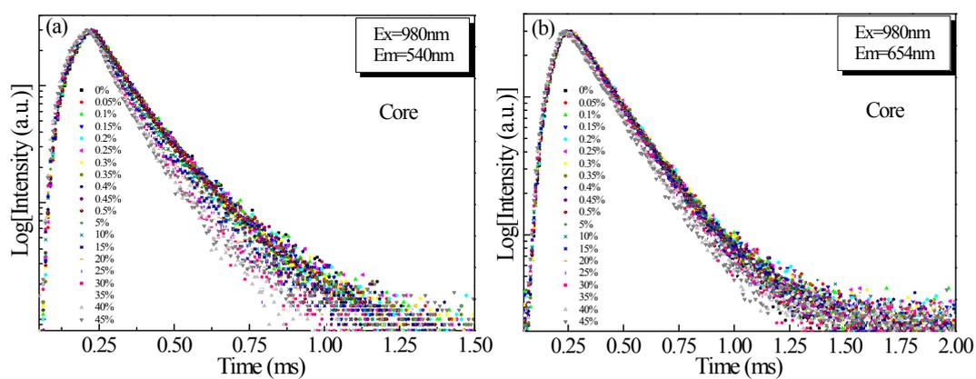
Figure S9 Water-content-dependent UC emission decay curves of (a)  $\text{Er}^{3+}: {}^2\text{H}_{11/2}, {}^4\text{S}_{3/2}$  emitting states ( $\lambda_{\text{em}} = 540 \text{ nm}$ ) and (b)  ${}^4\text{F}_{9/2}$  one ( $\lambda_{\text{em}} = 654 \text{ nm}$ ) for the core NCs under the excitation of 980 nm laser.
