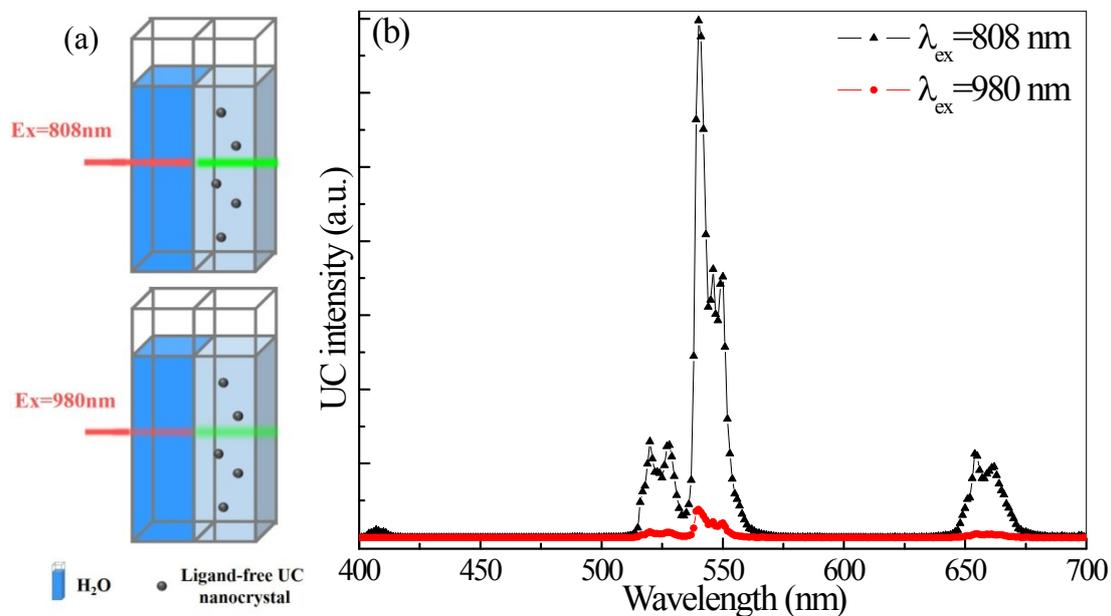
Figure S14 (a) Schematic illustrations of the noncontact method for measuring UC emission spectra under 808 nm or 980 nm laser excitation. (b) The corresponding UC emission spectra.
