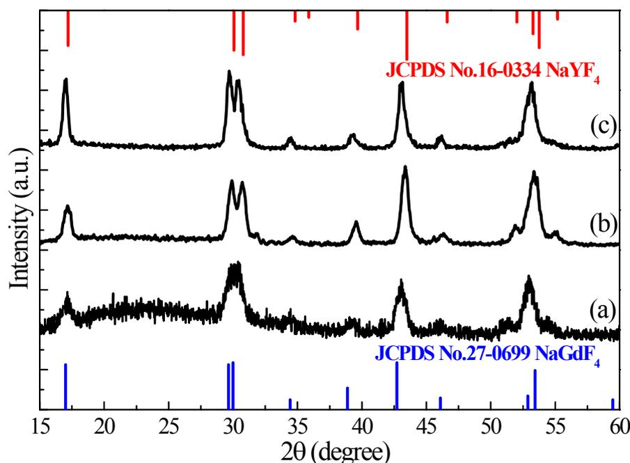
Figure S1 XRD patterns of (a) 20Yb/1Er:  $\text{NaGdF}_4$  core, (b) 20Yb/1Er:  $\text{NaGdF}_4@20\text{Yb}/10\text{Nd}$ :  $\text{NaYF}_4$  core-shell, (c) 20Yb/1Er:  $\text{NaGdF}_4@20\text{Yb}/10\text{Nd}$ :  $\text{NaYF}_4@\text{NaGdF}_4$  core-shell-shell samples. Bars represent standard hexagonal  $\beta\text{-NaYF}_4$  (JCPDS No. 16-0334) and  $\beta\text{-NaGdF}_4$  (JCPDS No. 27-0699) diffraction data, respectively.
