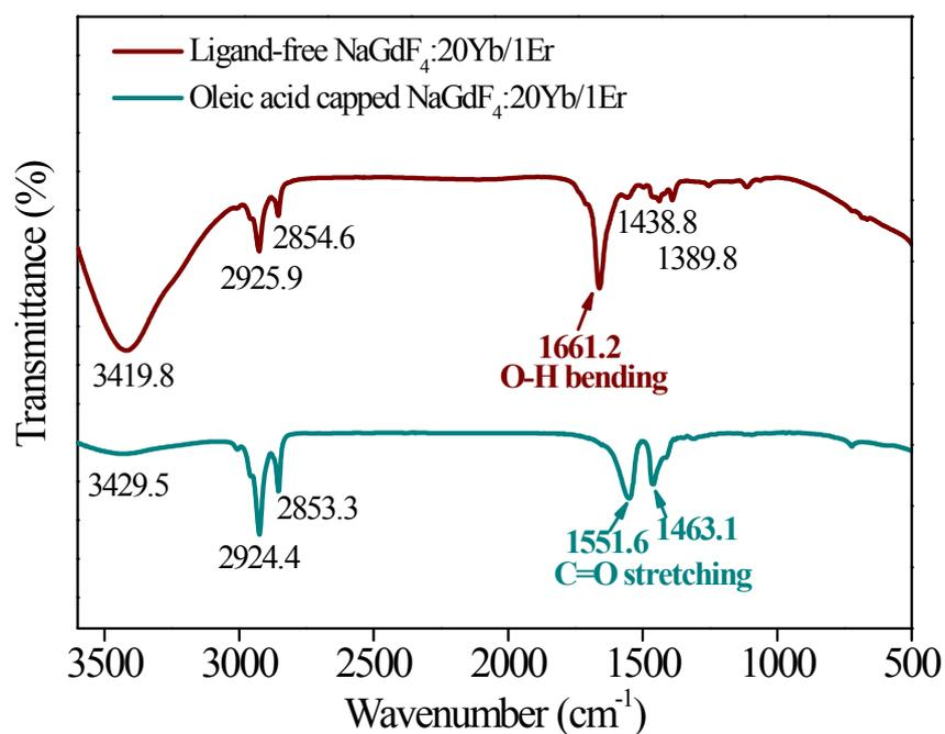
Figure S4 Fourier transform infrared spectroscopy (FTIR) of the oleic acid capped 20Yb/1Er: NaGdF<sub>4</sub> UCNCs (bottom) and the corresponding ligand-free sample (top).
