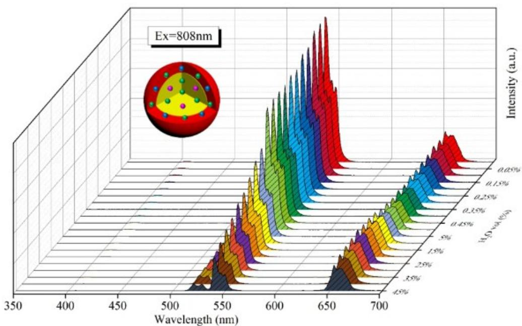
Figure S8 UC emission spectra of core-shell UCNCs dispersed in DMF solution with different water contents under the excitation of 808 nm laser.
