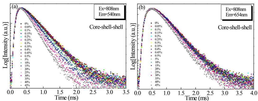
Figure S13 Water-content-dependent UC emission decay curves of (a)  $Er^{3+}: ^2H_{11/2}, ^4S_{3/2}$  emitting states ( $\lambda_{em} = 540$  nm) and (b)  $Er^{3+}: ^4F_{9/2}$  one ( $\lambda_{em} = 654$  nm) for the core-shell-shell NCs under the excitation of 808 nm laser.
