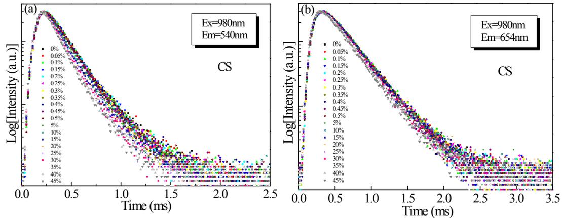
Figure S10 Water-content-dependent UC emission decay curves of (a)  $\text{Er}^{3+}$ :  $^2\text{H}_{11/2}$ ,  $^4\text{S}_{3/2}$  emitting states ( $\lambda_{\text{em}} = 540$  nm) and (b)  $^4\text{F}_{9/2}$  one ( $\lambda_{\text{em}} = 654$  nm) for the core-shell NCs under the excitation of 980 nm laser.
