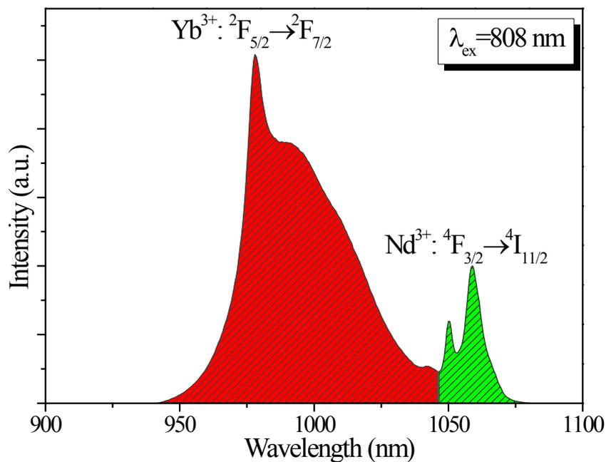
Figure S2 Photoluminescence spectrum of 20Yb/1Er:NaGdF<sub>4</sub>@20Yb/10Nd:NaYF<sub>4</sub>@NaGdF<sub>4</sub> core-shell-shell sample under the excitation of 808 nm laser.
