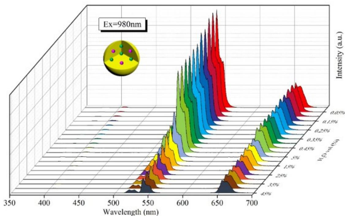
Figure S5 UC emission spectra of core UCNCs dispersed in DMF solution with different water contents under the excitation of 980 nm laser.
