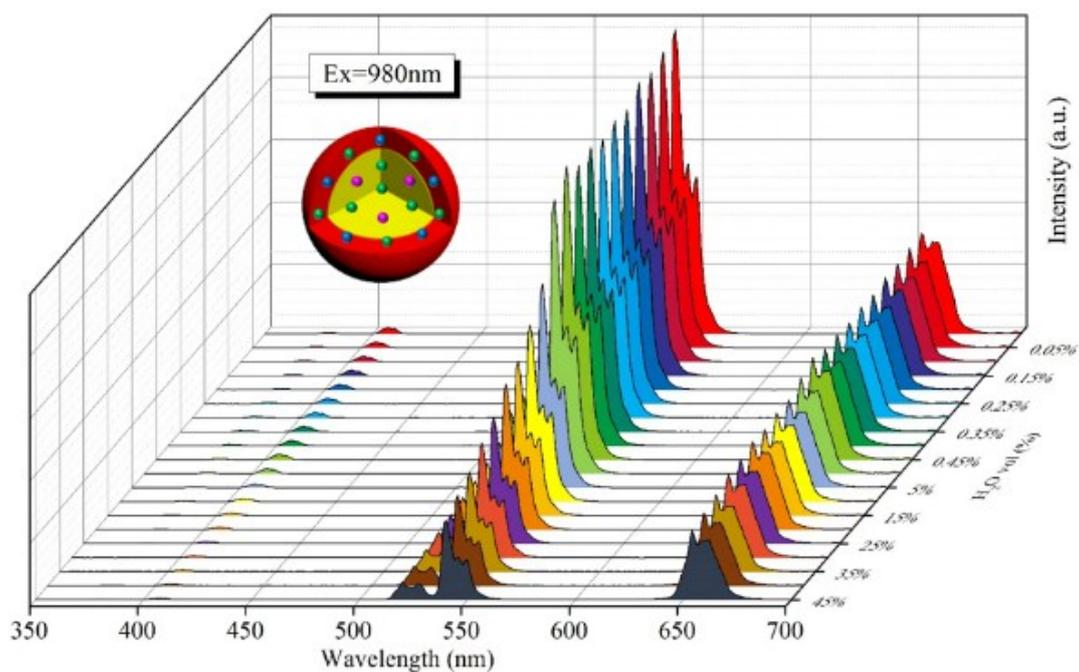
Figure S6 UC emission spectra of core-shell UCNCs dispersed in DMF solution with different water contents under the excitation of 980 nm laser.
