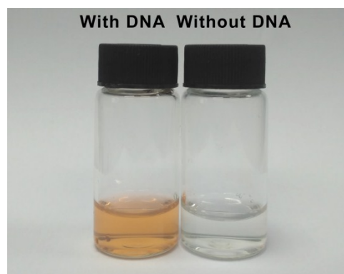
Figure S2. The SSDG NPs and SG loaded gelatin NPs with DNA after 72 hours dialysis in pure water.
