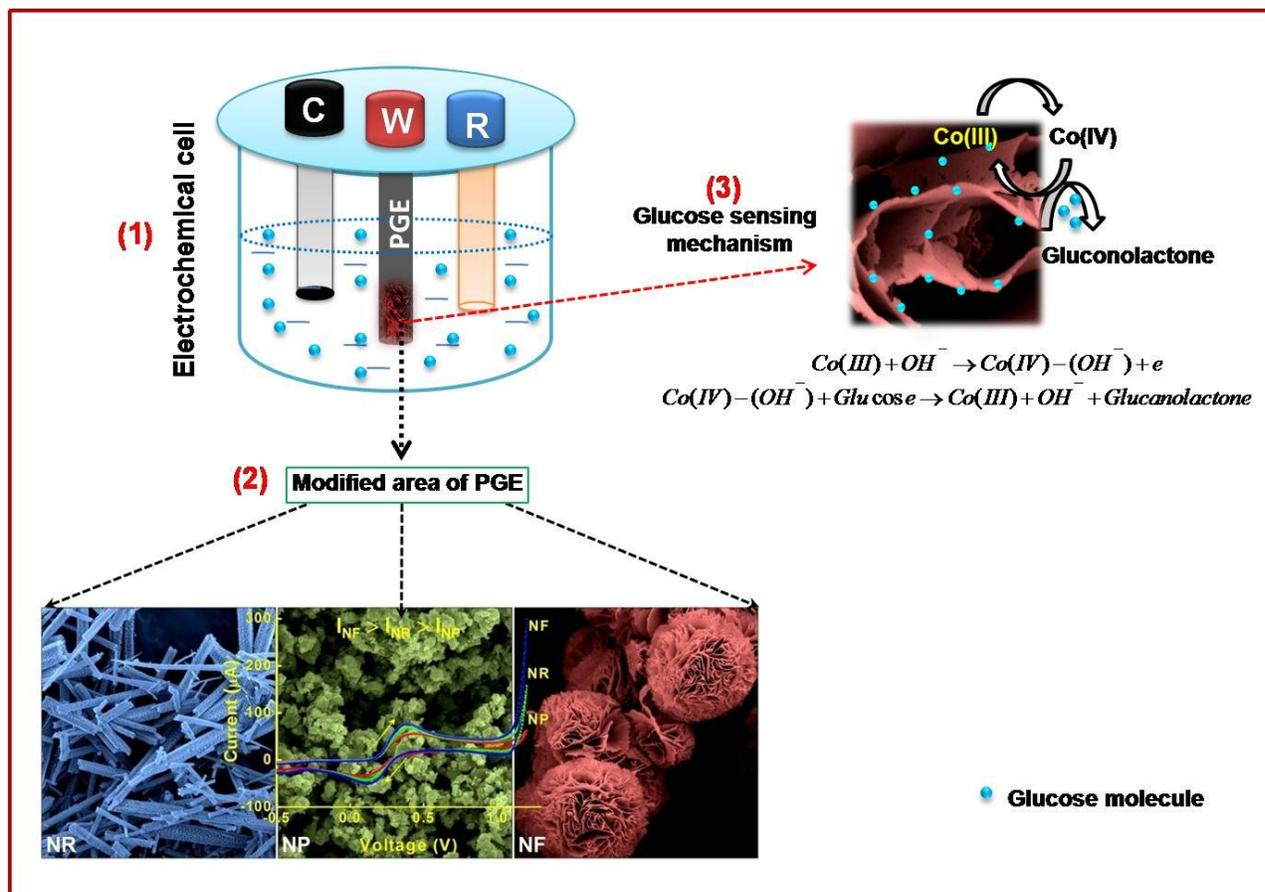
**Scheme S 1: Shape-specific electrocatalytic oxidation mechanism of glucose.**
