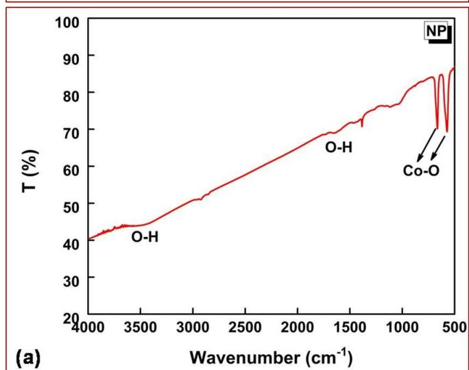
Fig. S1 FTIR spectra of cobalt oxide nanostructures.
