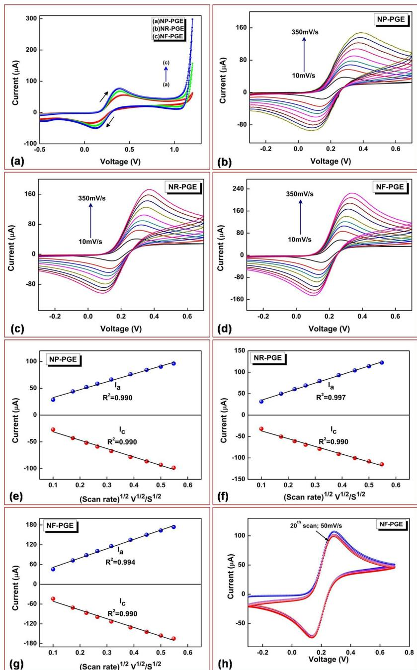
**Fig. S2:** (a) CV of the prepared electrodes in 1M aqueous KCl solution containing 5mM/L  $K_3Fe(CN)_6$  at a scan rate of 50mV/s. (b), (c) and (d) represents CV scans at various scanning potentials for modified electrodes, (e), (f) and (g) Shows the linear fitted plots of peak currents against square root of scan rates for modified electrodes. (h) Repeatability of CONF-PGE for 20 CV runs at 50mV/s.
