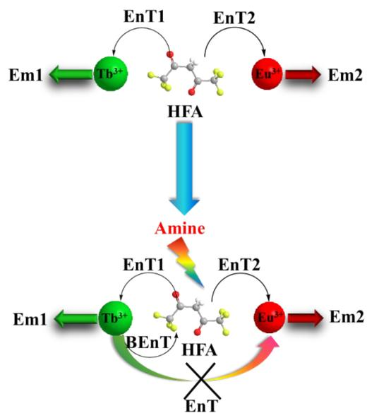
**Scheme S1** Detailed process of energy transfer from ligand HFA to Tb<sup>3+</sup> and Eu<sup>3+</sup> with the stimulation of amine vapors (EnT: energy transfer, BEnT: energy back transfer).
