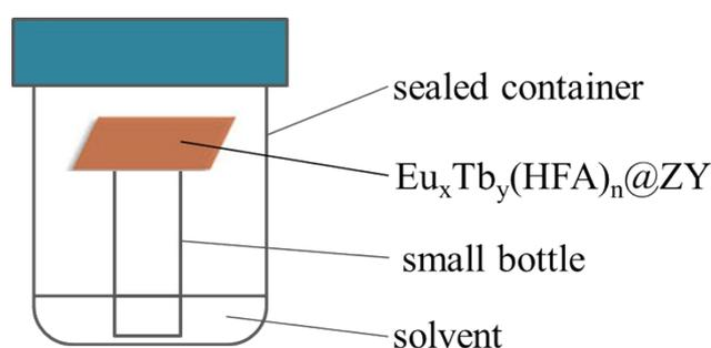
**Figure S18** Diagram of the experimental setup for exposing  $\text{Eu}_x\text{Tb}_y(\text{HFA})_n@ZY$  to various amine solvent vapors.
