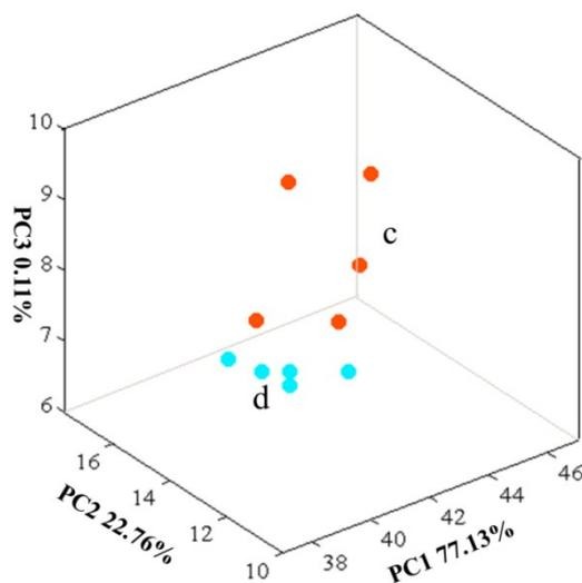
**Figure S10** The enlarged three dimensional PCA score plot for c (Butylamine) and d (1,3-Propanediamine) derived from the luminescence data.
