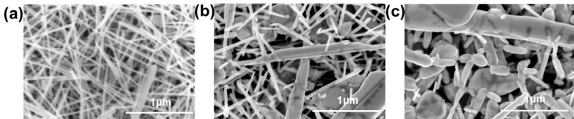
Fig. S2 Microstructure of (a) silver nanowire film annealed at 150 °C (b) silver nanowire film annealed at 200 °C (c) silver nanowire film annealed at 230 °C
