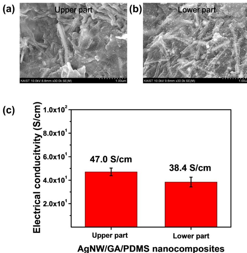
Fig. S7 Microstructures of (a) upper part (b) lower part in AgNW (0.7 vol.)/GA/PDMS nanocomposites (c) Electrical conductivity as parts of the AgNW (0.7 vol.)/GA/PDMS nanocomposites
