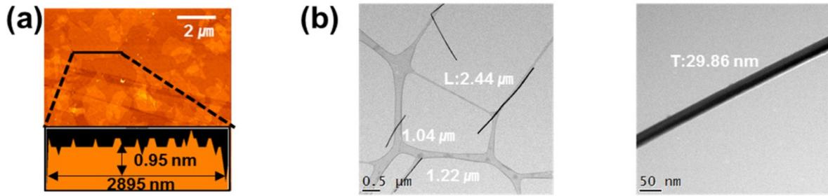
Fig. S1 (a) AFM images of graphene oxides and their thickness with lateral size (b) TEM images of silver nanowires and their thickness with length
