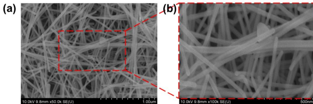
Fig. S3 Microstructure of (a) optically treated silver nanowire films and (b) their magnified image
