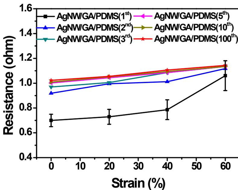
Fig. S9 Electrical resistance changes of AgNW/GA/PDMS nanocomposites according to stretching cycles
