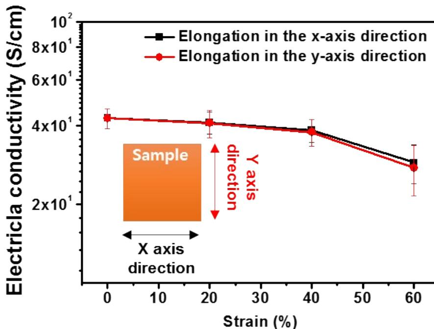
Fig. S8 Electrical conductivity curve of AgNW/GA/PDMS nanocomposites with strain direction
