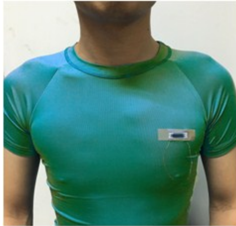
Figure S10. Photographs showing the CSG-based stain sensor attached on a running tights for monitoring respiration..
