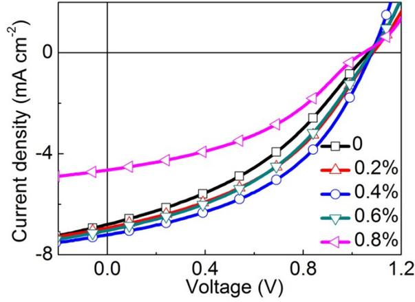
Fig. S3. J-V curves of the OSC devices based on  $p$ -DTS(FBTTh<sub>2</sub>)<sub>2</sub>:P-BNBP-T blend (2:1, w/w) processed with different DIO content and thermal annealing at 80 °C.
