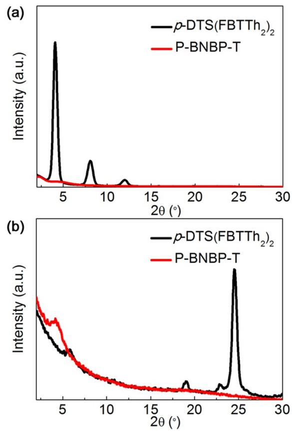
Fig. S4. GI-XRD patterns of the pure  $p$ -DTS(FBTTh<sub>2</sub>)<sub>2</sub> film and the pure P-BNBP-T film:
