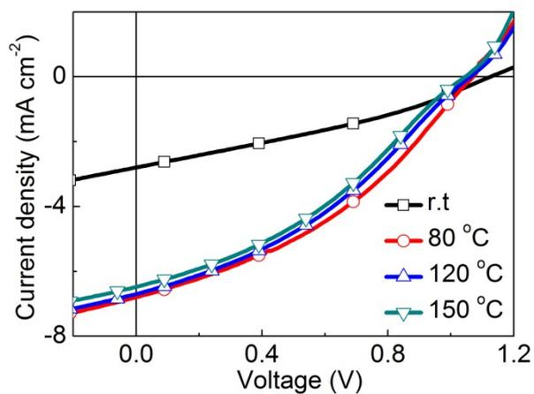
Fig. S2. J-V curves of the OSC devices based on  $p$ -DTS(FBTTh<sub>2</sub>)<sub>2</sub>:P-BNBP-T blend (2:1, w/w) annealing at different temperatures.
