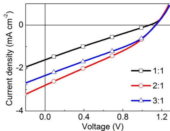
Fig. S1.  $J$ - $V$  curves of the OSC devices based on  $p$ -DTS(FBTTh<sub>2</sub>)<sub>2</sub>:P-BNBP-T blend with different weight ratios.
