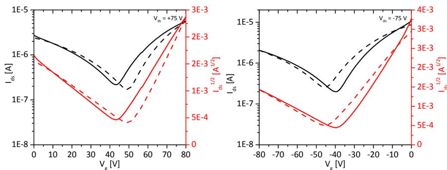
Figure S6: OFET output (top) and transfer (bottom) characteristics: p-channel operation (left) and n-channel operation (right) of P(TPD-TPF<sub>2</sub>T) after thermal annealing. Solid lines represent forward scans and dashed lines reversed scans.
