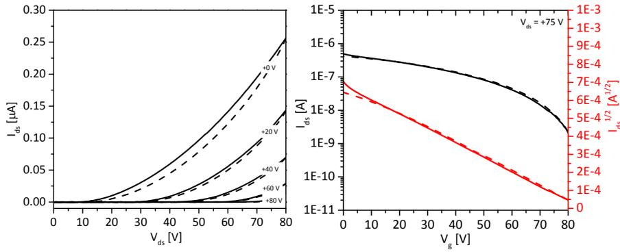
Figure S4: OFET output (left) and transfer (right) characteristics: n-channel operation of P(TPD-TPT) in the as cast state. Solid lines represent forward scans and dashed lines reversed scans.
