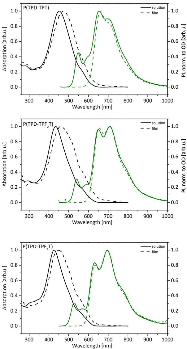
Figure S3. UV-Vis and photoluminescence spectra in solution and thin films for each PTPD.
