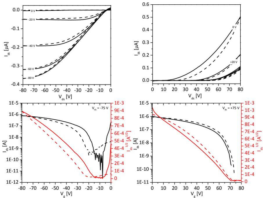
Figure S5: OFET output (top) and transfer (bottom) characteristics: p-channel operation (left) and n-channel operation (right) of P(TPD-TPF<sub>2</sub>T) in the as cast state. Solid lines represent forward scans and dashed lines reversed scans.
