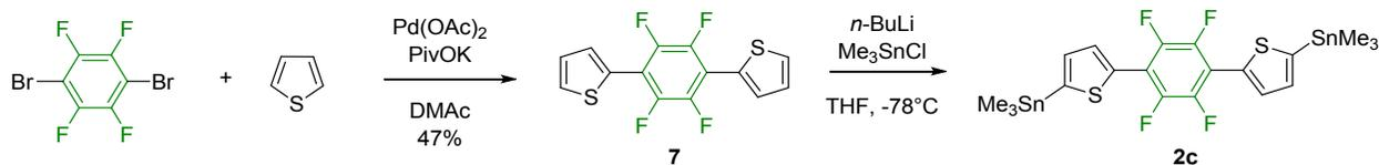
Scheme S2. Synthesis of the TPF<sub>4</sub>T monomer.
