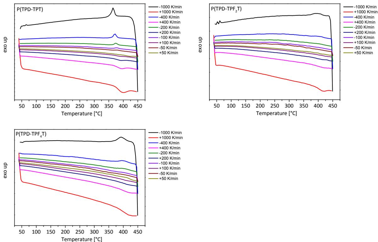
Figure S2. Flash-DSC analysis of the PTPDs with scanning rates from 50-1000 K/min.
