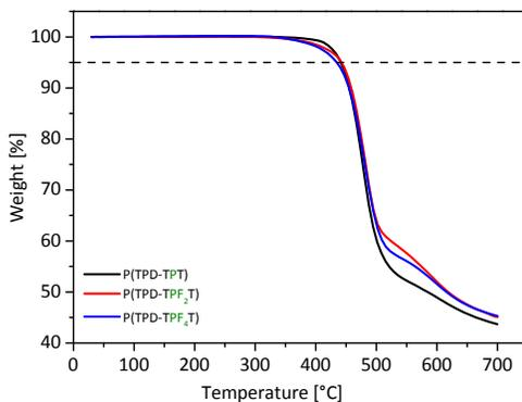
Figure S1. Thermogravimetric analysis of the PTPDs with the decomposition onset ( $T_{5\%}$ ).
