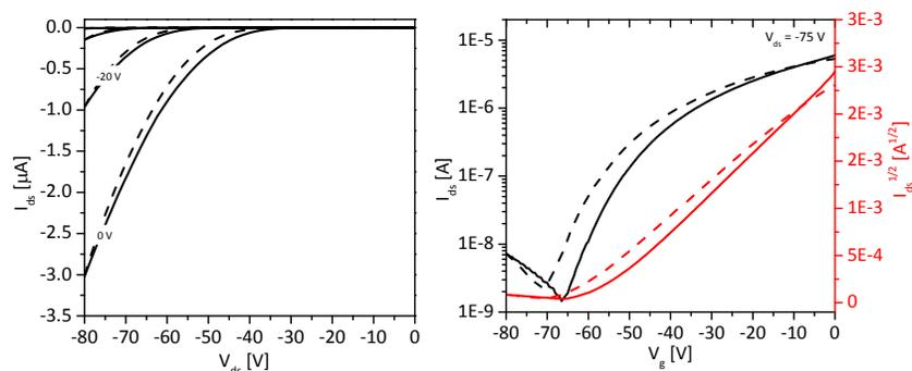
Figure S7: OFET output (left) and transfer (right) characteristics: p-channel operation of P(TPD-TPF<sub>4</sub>T) after thermal annealing. Solid lines represent forward scans and dashed lines reversed scans.
