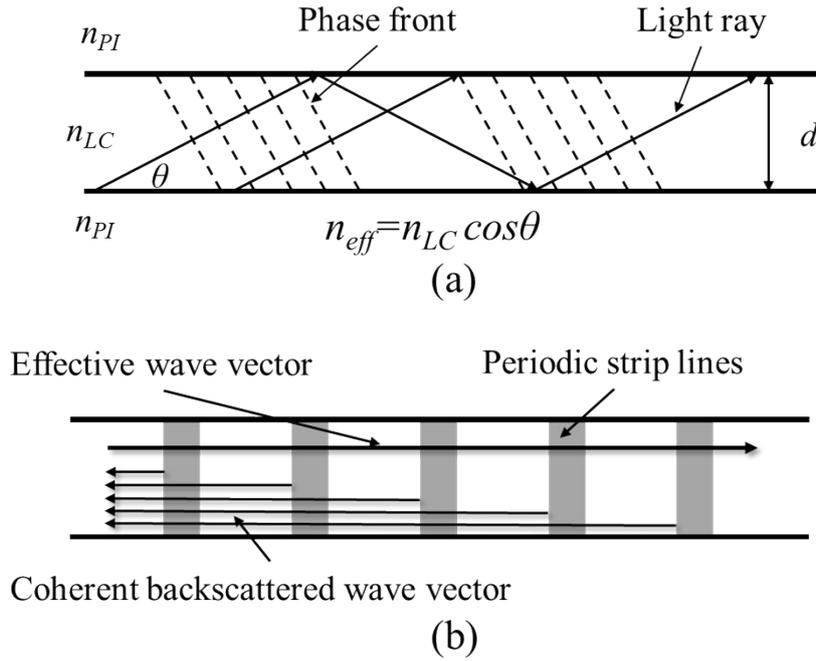
**Fig. S2** Illustration for the mode selection mechanism of the high-order DFB based on a waveguide structure. (a) the waveguide configuration; (b) the high-order DFB configuration.
