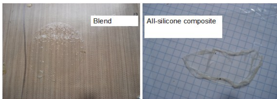
Figure S1: Cl-modified silicone mixed with PDMS and cross-linked together (left) versus PDMS –polar particles composite film (right)
