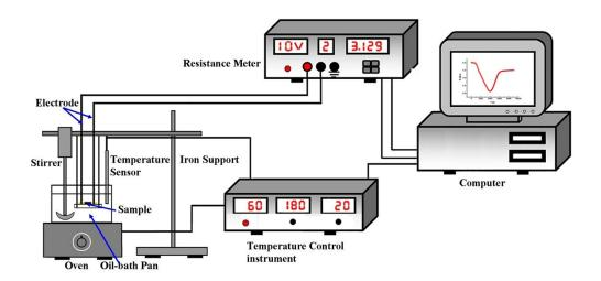
Fig. S1. The schematic figure of the equipment for temperature-resistivity test.
