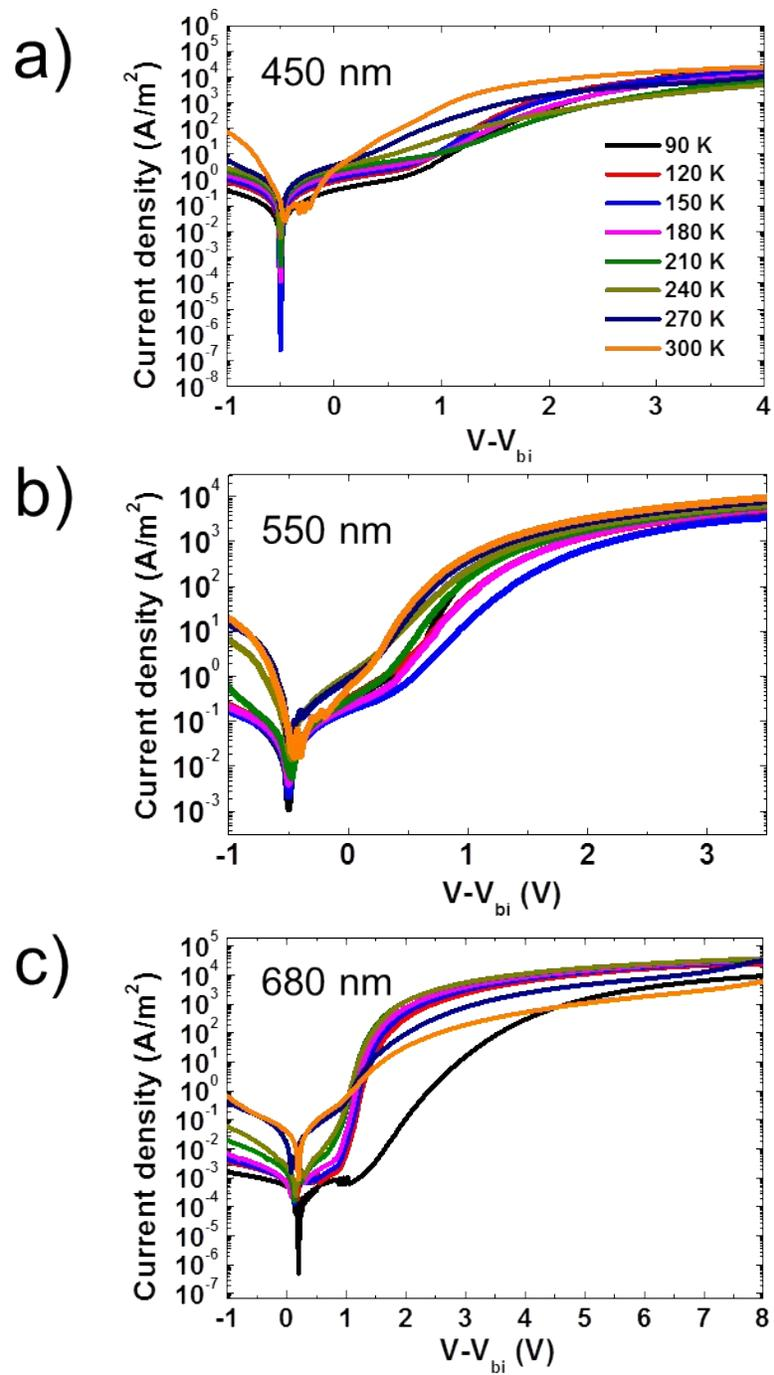
**Figure S1.** (a)-(c) Temperature-dependent current density versus voltage characteristics in semi-logarithm scale of MAPbI<sub>3</sub> hole-only devices with various  $L$  scanned in the downward direction.
