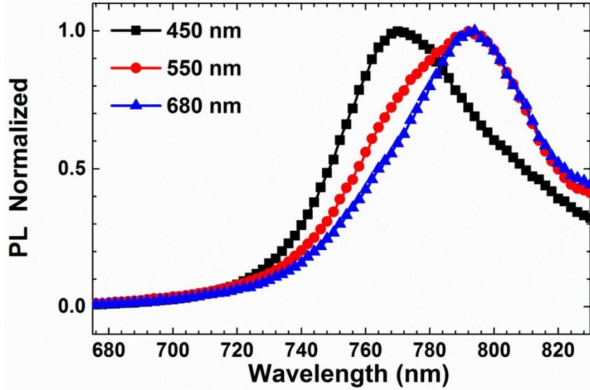
**Figure S2.** Steady-state photoluminescence spectroscopy of MAPbI<sub>3</sub> films with different  $L$ .
