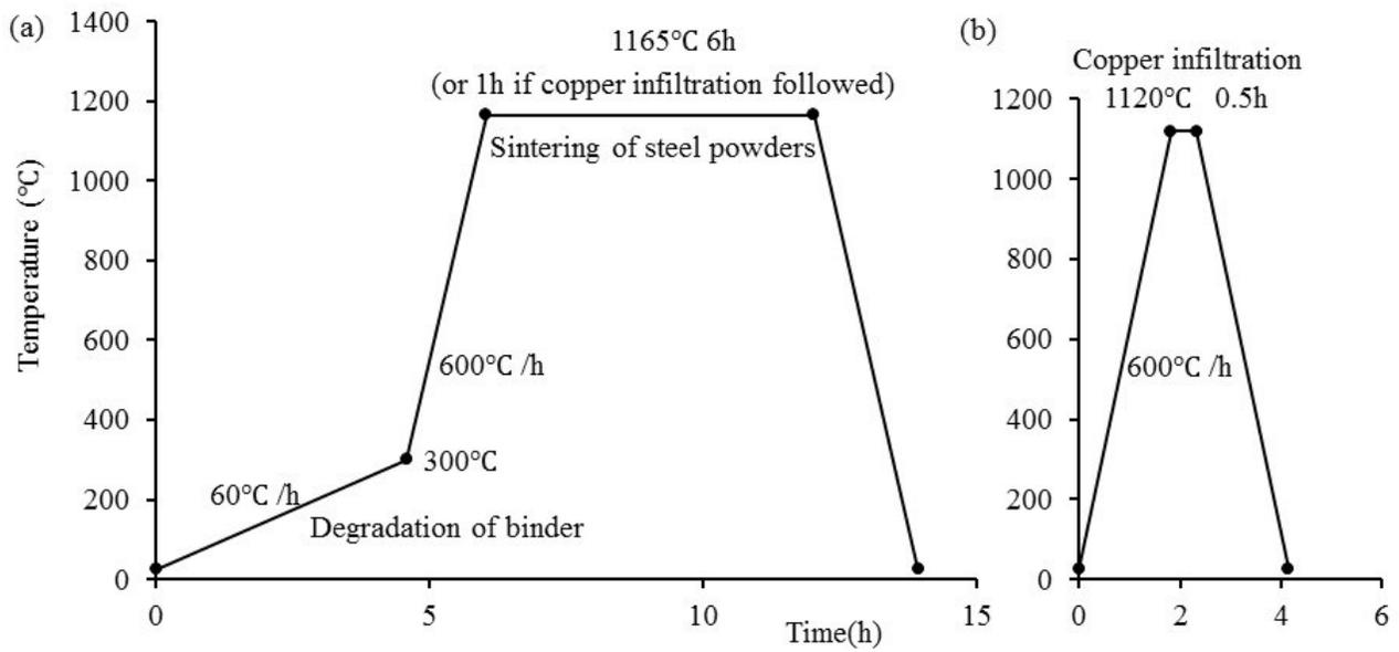
**Figure S6.** Temperature profiles using during sintering and copper infiltration. Debinding starts from 25 °C to 300 °C with a heating rate of 60 °C/h. Then the temperature is raised up to 1165 °C with a heating rate of 600 °C/h and held at 1165 °C for 6h for sintering. For copper infiltration, the temperature is raised up to 1120 °C and held for 0.5 h, then cooled down to the room temperature.
