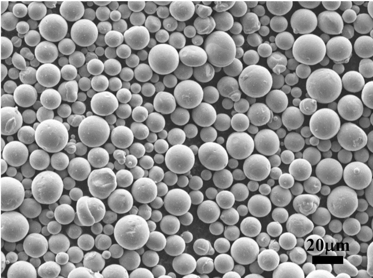
**Figure S1.** Secondary electron micrograph of HAS powder particles ( $\leq 20 \mu\text{m}$ ).
