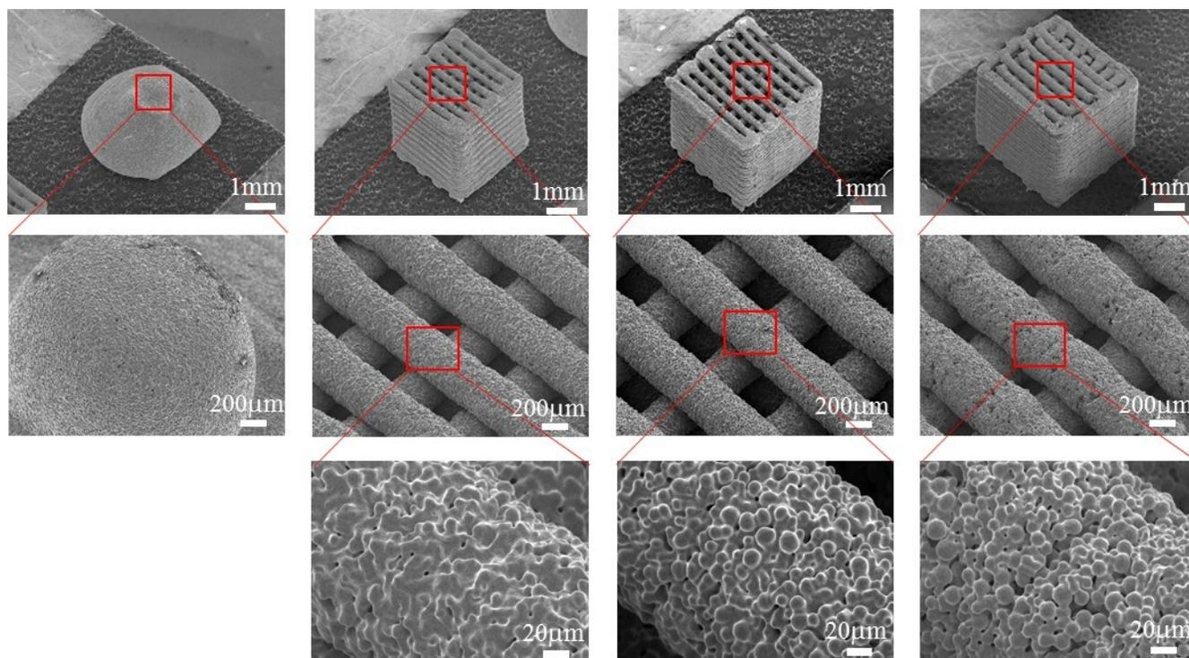
**Figure S3.** SEM images of sintered 20-layers scaffolds of different concentrated inks (85, 90, 95, 98 wt.%) (first row from left to right) and their close-up view images (middle and bottom rows). After sintering, the polymer is burned away and the HAS microparticles are sintered together. The filaments of 90, 95 and 98 wt.% scaffold keep their shapes and align well, while the 85 wt.% ink printed scaffold collapses during sintering and the surface of 98 wt.% scaffold is rough.
