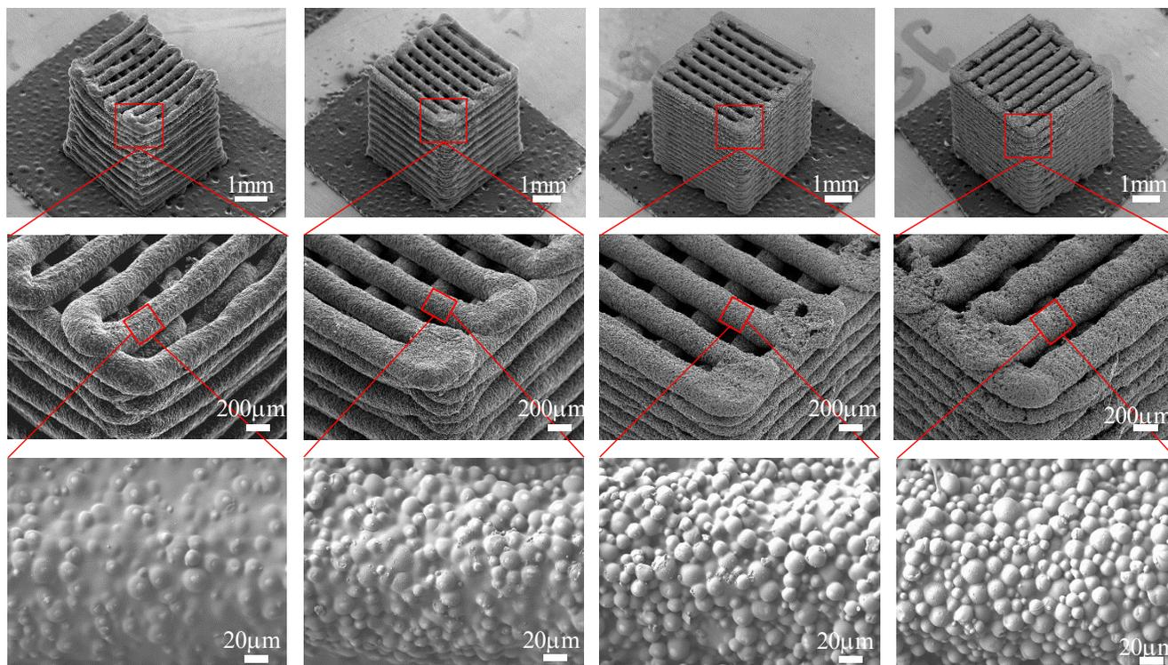
**Figure S2.** SEM images of as-printed 20-layers scaffolds of different concentrated inks (85, 90, 95, 98 wt.%) (first row from left to right) and their close-up view images (middle and bottom rows). The HAS microparticles are covered and bonded by the polymer. The filaments of all four scaffolds align well. However, the 85 wt.% scaffold distorts and the surface of the 98 wt.% scaffold is rough.
