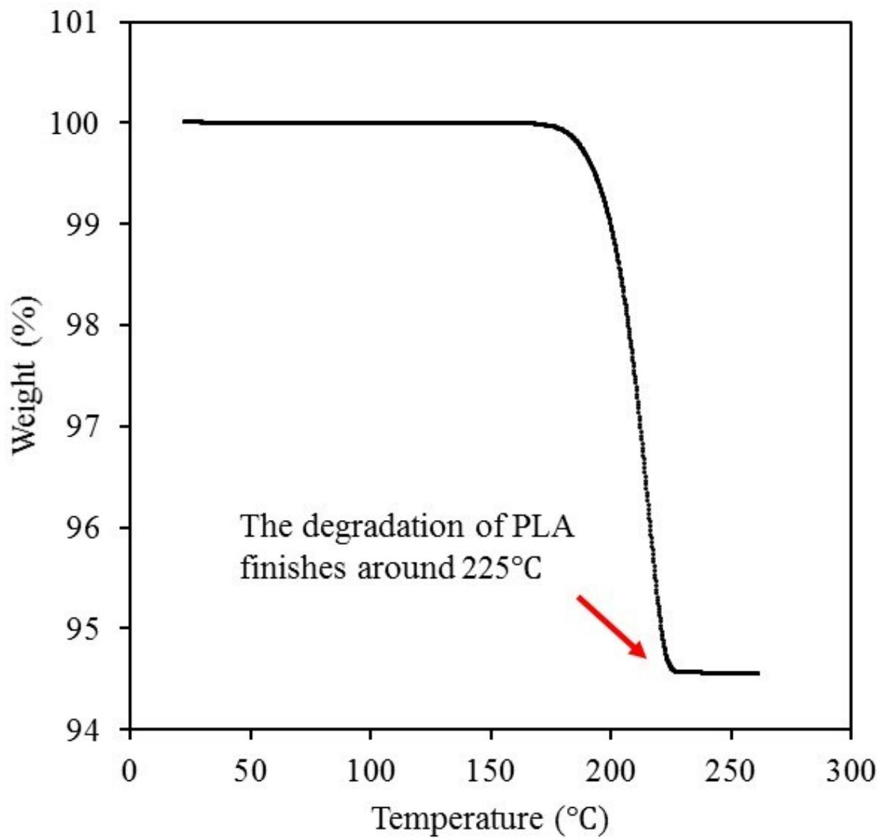
**Figure S5.** TGA results of 95 wt.% HAS/PLA scaffold. The temperature is raised from 20 °C to 500 °C at a rate of 1 °C/min (the same heating rate as the sintering process). The degradation of PLA finishes before 225 °C.
