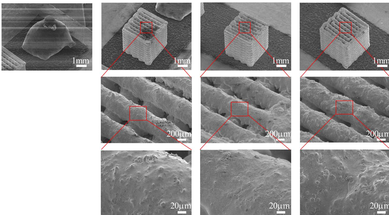
**Figure S4.** SEM images of copper infiltrated 20-layers scaffolds of different concentrated inks (90, 95, 98 wt.%) (first row from left to right) and their close-up view images (middle and bottom rows). Melted copper infiltrated into the sintered filaments. Some excess copper is left on the top of the scaffold.
