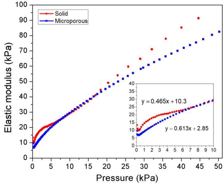
Fig. S2. Elastic modulus of the dielectric materials as a function of pressure. The microporous PDMS has lower elastic modulus (as seen from the inset) at low pressures and it increases slowly with pressure as compared to solid PDMS.
