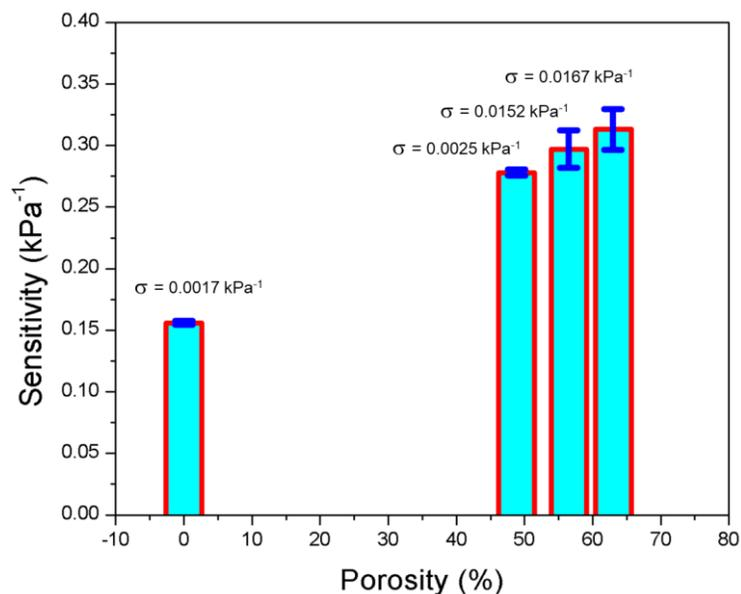
Fig. S4. Sensitivities and their error deviation from mean value for different values of glucose to PDMS composition. Higher value of glucose to PDMS ratio,  $v_g/v_p$  can give better sensitivity but resulted inconsistency in sensitivity values since the microporous PDMS suffered from unstable fiber morphology.
