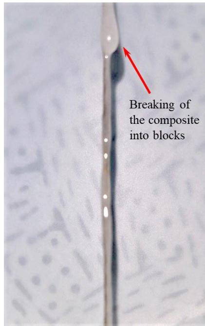
Fig. S3. Unstable morphology corresponding to drops sliding down the fiber. At high concentration of glucose particles (glucose/PDMS volume ratio of 1.3), due to a high zero shear viscosity, the composite hardly or couldn't flow along the fiber. The continuous liquid thread breaks into gel-like blocks.
