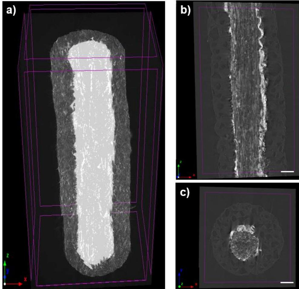
*Fig. S1. X-ray microcomputed tomography (micro-CT) images a) showing 3-dimensional view of the microporous PDMS coated on the conductive fiber, b) vertical cross-section from the center and c) horizontal cross-section showing micropores. The scale of white bar represents 200  $\mu\text{m}$ . Skyscan 1172 was used to take the micro-CT images.*
