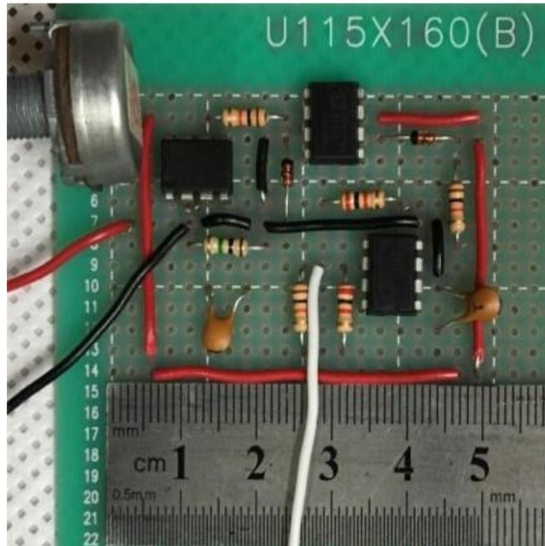
*Fig. S7. PCB layout of the capacitance detection circuit for the measurement of output voltage.*
