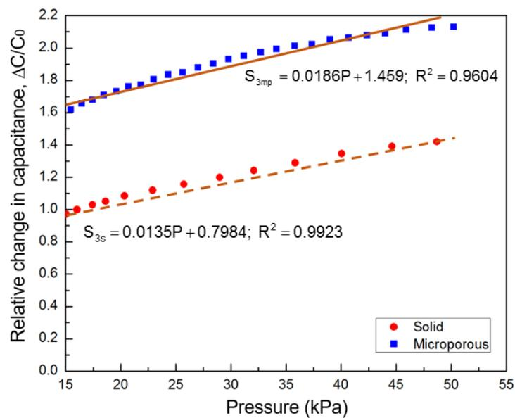
Fig. S5. Relative capacitance change ( $\Delta C/C_0$ ) in response to external pressure for  $>15$  kPa. In the higher pressures, the contact area induces lower effective stress because pores appeared to be completely closed. Although the sensitivity in this region is lower than that of the first region, but higher than solid PDMS-coated feature.
