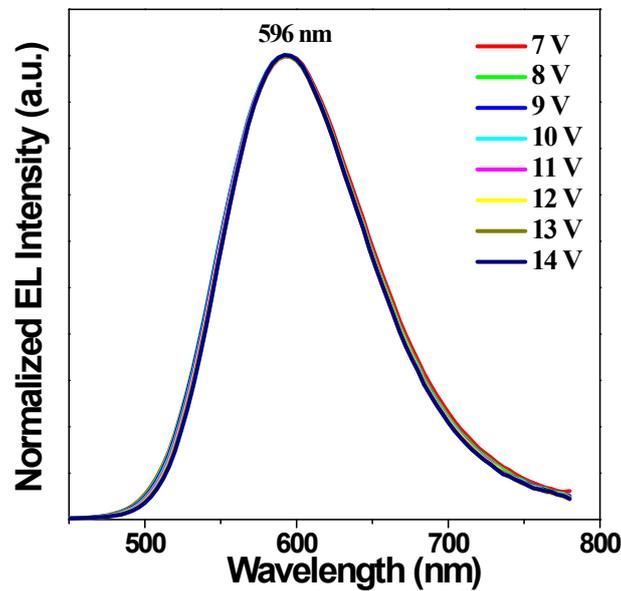
**Figure S2** The spectra of the device at different voltages.
