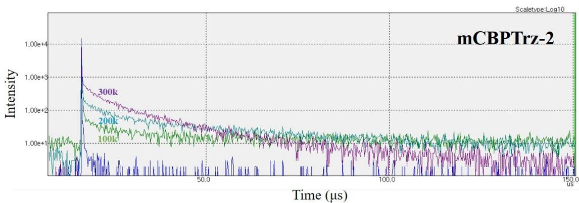
**Figure S5.** PL decay curves of mCBPTrz-1 and mCBPTrz-2 measured at various temperatures.
