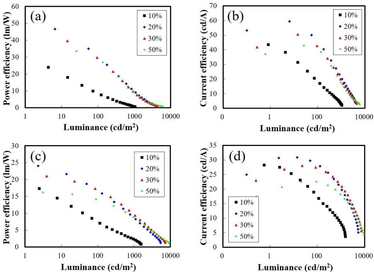
**Figure S4.** Power and current efficiencies (a), (b) for mCBPTrz-1 and (c), (d) for mCBPTrz-2.
