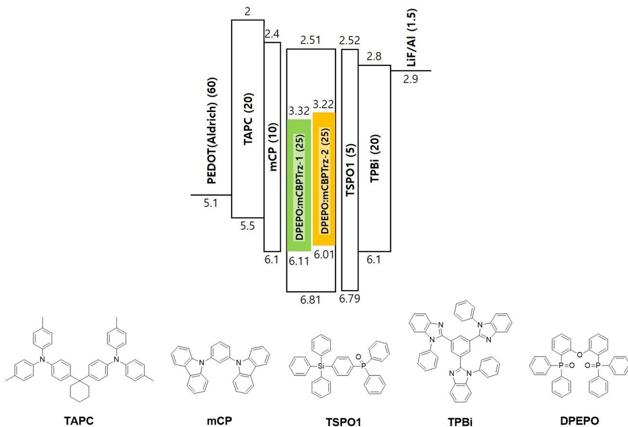
**Figure S3.** Energy level diagram and chemical structure of materials.
