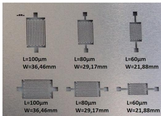
**Figure S1.** Scheme of a substrate including six OFETs of variable dimensions.
