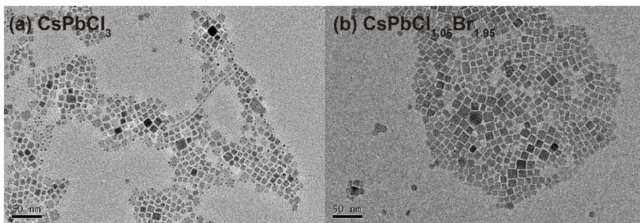
Fig. S3 TEM images of (a)  $\text{CsPbCl}_3$  QDs; (b)  $\text{CsPbCl}_{1.05}\text{Br}_{1.95}$  QDs obtained by in situ ion exchange method.
