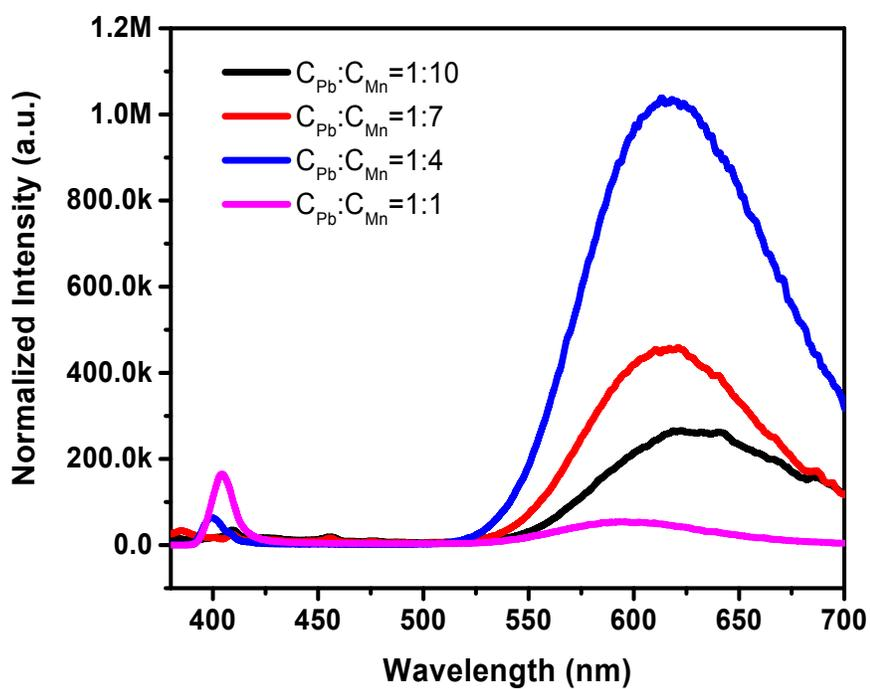
Fig. S4 Photoluminescence spectra of  $\text{CsPb}_x\text{Mn}_{1-x}\text{Cl}_3$  QDs synthesized with different Pb-to-Mn ratio.
