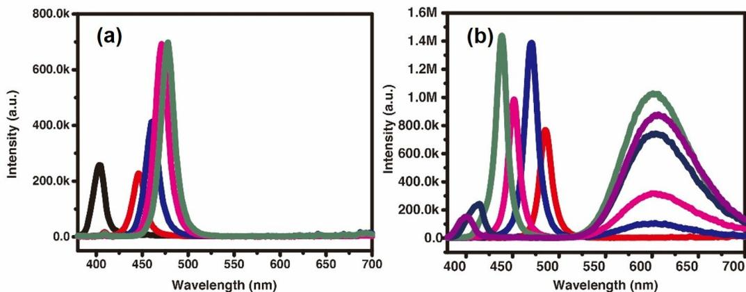
Fig. S6 Photoluminescence spectra of the corresponding (a) CsPb(Cl<sub>x</sub>Br<sub>1-x</sub>)<sub>3</sub> QDs and (b) Cs(Pb<sub>x</sub>Mn<sub>1-x</sub>)(Cl<sub>y</sub>Br<sub>1-y</sub>)<sub>3</sub> QDs obtained by in situ ion exchange method.
