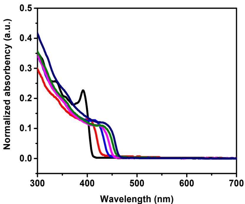
Fig. S7 UV-visible optical absorption of the corresponding CsPb(Cl<sub>x</sub>Br<sub>1-x</sub>)<sub>3</sub> QDs obtained by in situ ion exchange method.
