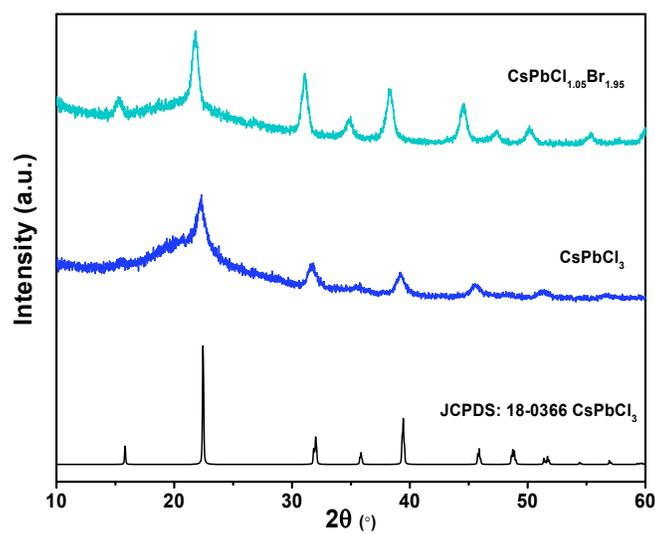
Fig. S2 XRD patterns of  $\text{CsPbCl}_3$  QDs and  $\text{CsPbCl}_{1.05}\text{Br}_{1.95}$  QDs. The latter one prepared by the in situ ion exchange method.
