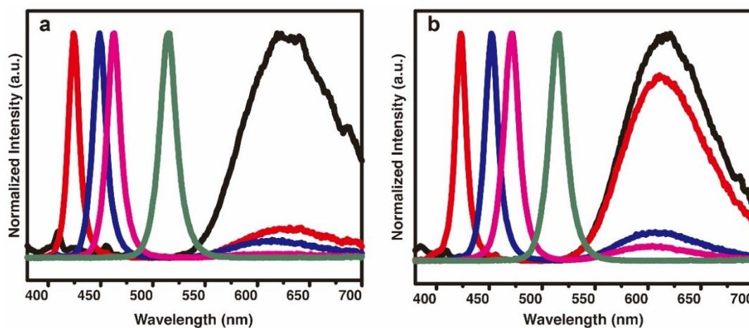
Fig. S5 Photoluminescence spectra of the corresponding  $\text{Cs}(\text{Pb}_x\text{Mn}_{1-x})(\text{Cl}_y\text{Br}_{1-y})_3$  QDs obtained by in situ ion exchange method with different end member of  $\text{CsPb}_x\text{Mn}_{1-x}\text{Cl}_3$ . (a)  $\text{CsPb}_{0.64}\text{Mn}_{0.36}\text{Cl}_3$  (b)  $\text{CsPb}_{0.79}\text{Mn}_{0.21}\text{Cl}_3$ .
