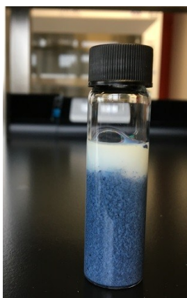
Fig S2 The combination of NP1 and rGO ink demonstrates incompatibility of these two inks.
