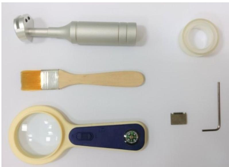
**Fig. S6** Tools used to test adhesion of copper patterns.
