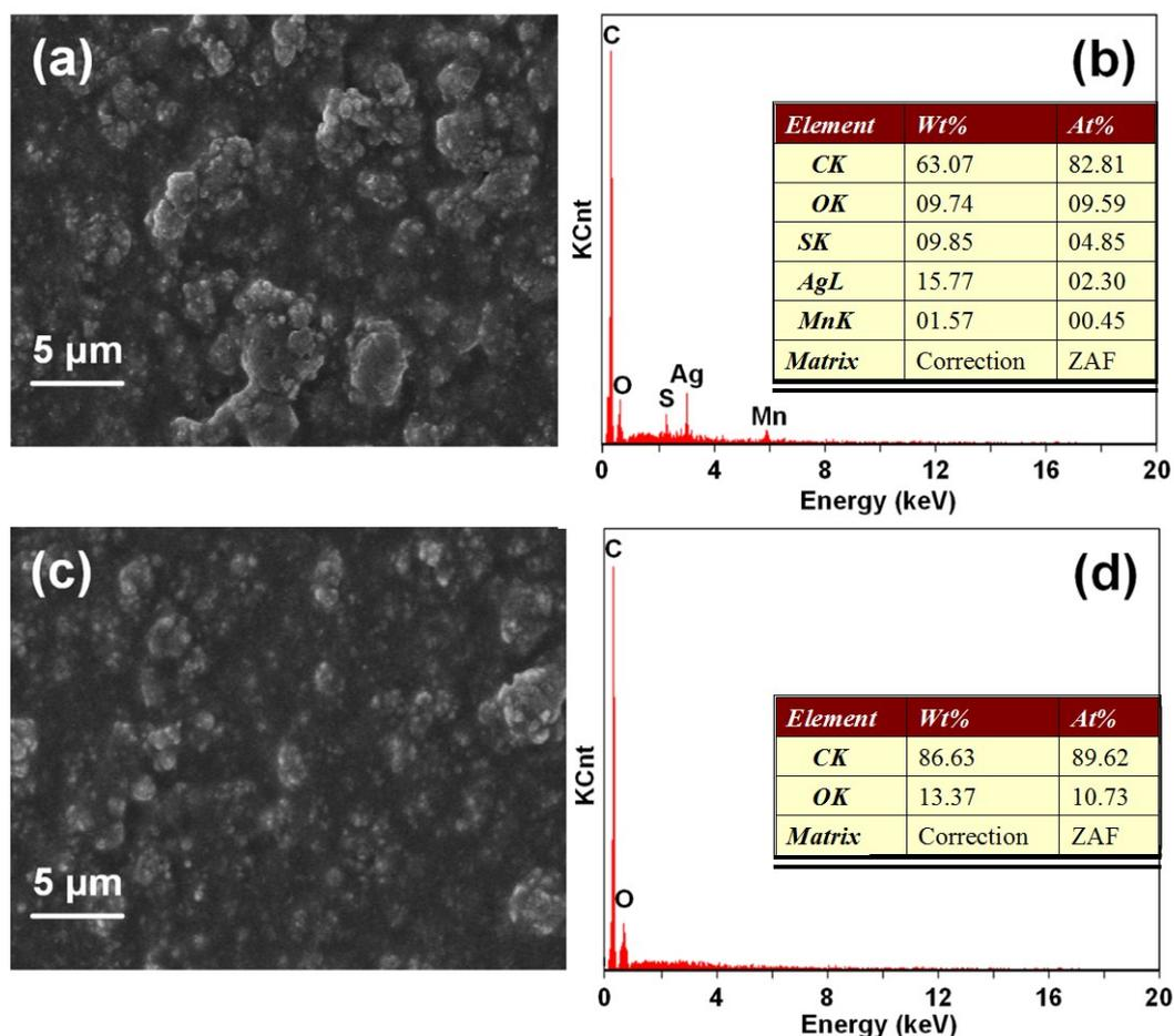
**Fig. S3** SEM images and EDS spectra of (a), (b) modified and (c), (d) pristine substrate after immersing  $\text{AgNO}_3/\text{C}_2\text{H}_5\text{OH}$  solution and ultrasonic washing.
