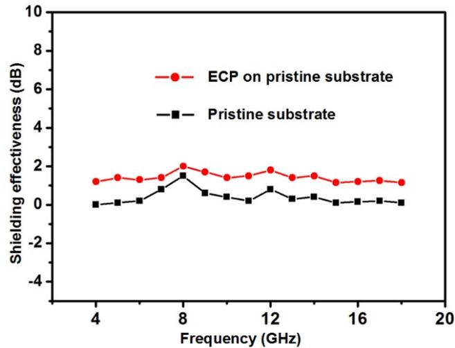
Fig. S8 The variation in EMI shielding effectiveness of pristine and ECP on pristine epoxy resin substrate range from 4 GHz to 18GHz.
