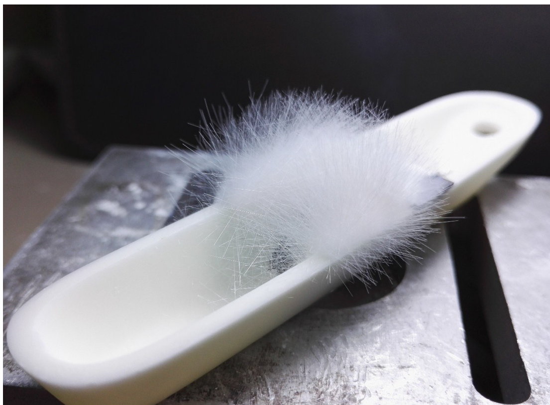
Figure S8. Individual Sb-doped ZnO microwires were synthesized by a catalyst-free, vapor-solid process via chemical vapor deposition (CVD).
