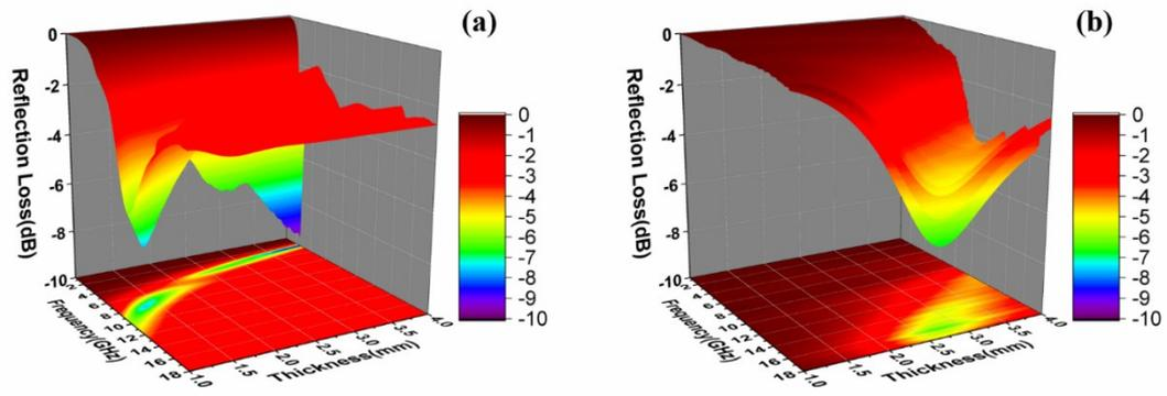
**Fig. S3** 3D RL plots of (a)P-SWCNTs and (b) 31.4%F-SWCNTs versus frequency ranging from 0.5 to 18GHz and thickness ranging from 1 to 4 mm.
