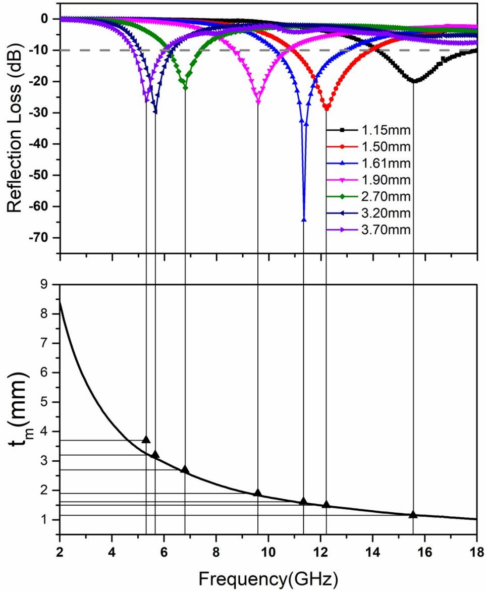
Fig. S4 Reflection loss curves and dependence of matching thickness versus matching frequency with  $n=1$
