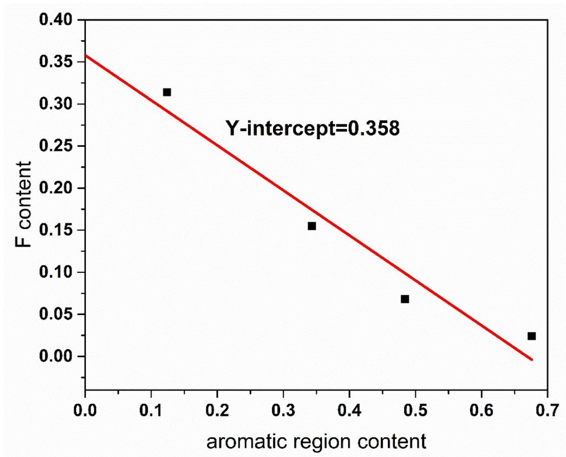
**Fig. S1** plot of F content versus aromatic region content of F-SWCNT with various F content.
