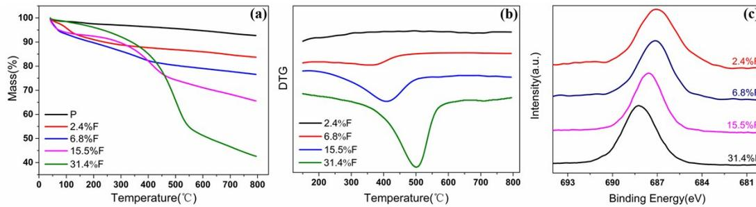
**Fig. S2** (a)TGA and (b)DTG and (c)F 1s/XPS spectra curves of F-SWCNTs with various F-content.
