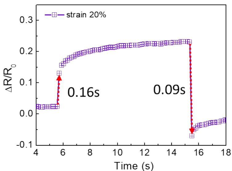
**Figure S4.** The strain-response showing rise and decay time of Zn<sub>2</sub>GeO<sub>4</sub>@PPy NW aerogels under 20% strain.
