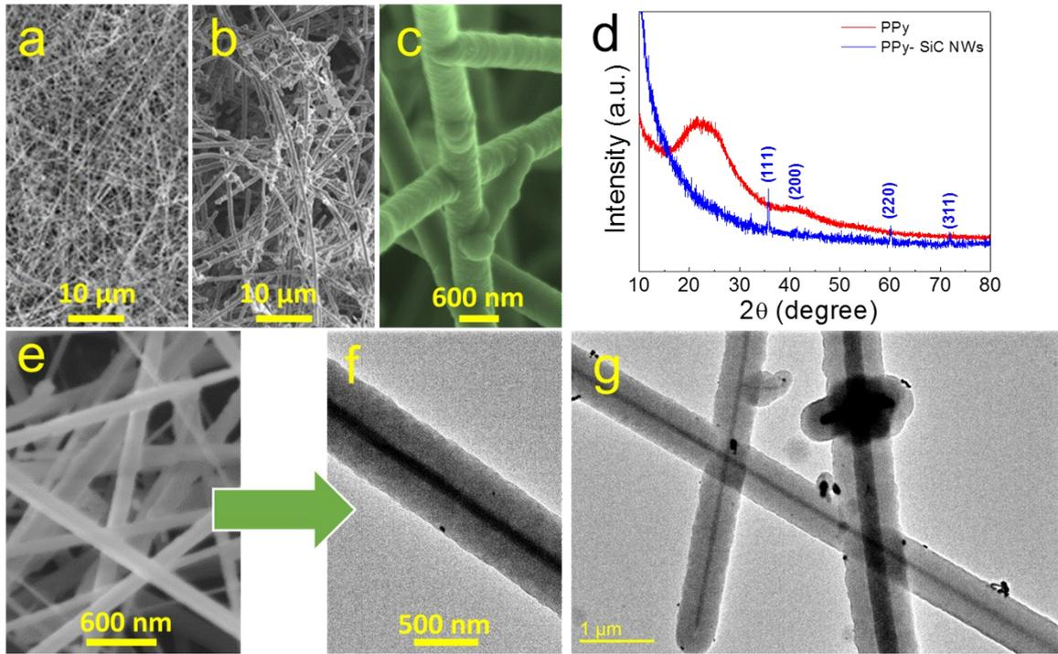
**Figure S2.** Microstructure of SiC NWs and PPy- SiC NW aerogels. (a) Scanning Electron Microscope (SEM) and Transmission Electron Microscope (TEM) (e) images of SiC NWs. (b) Low resolution and (c) High resolution SEM images of PPy- SiC NW aerogels. (d) XRD spectra of PPy-SiC NW hybrid aerogels and PPy. (f-g) TEM images of PPy-SiC NW aerogels
