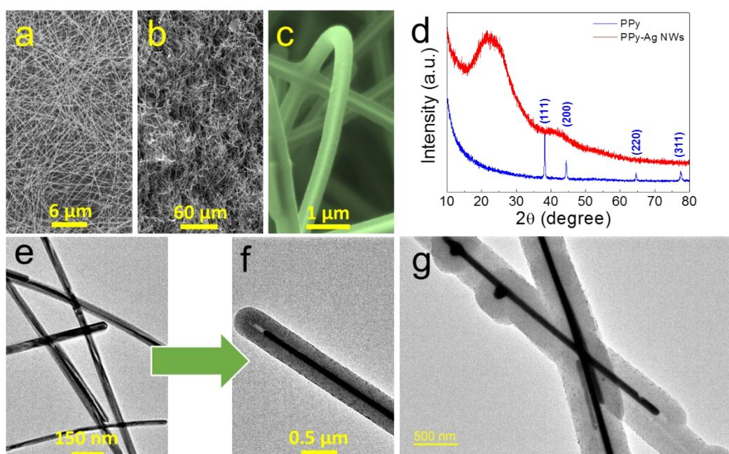
**Figure S1.** Microstructure of Ag NWs and PPy-Ag NW aerogels. (a) Scanning Electron Microscope (SEM) and Transmission Electron Microscope (TEM) (e) images of Ag NWs. (b)
