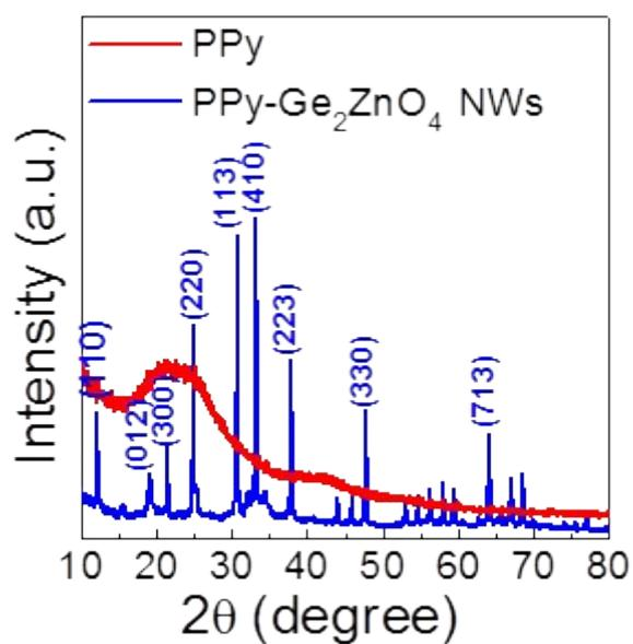
**Figure S3.** XRD spectra of PPy-Zn<sub>2</sub>GeO<sub>4</sub> NW hybrid aerogels and PPy.
