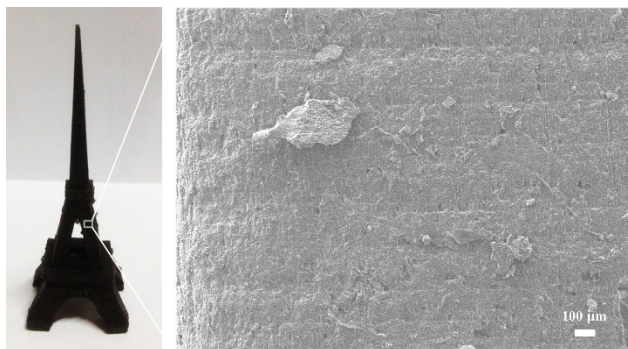
Figure S6. The surface morphology of the printed object investigated by SEM.
