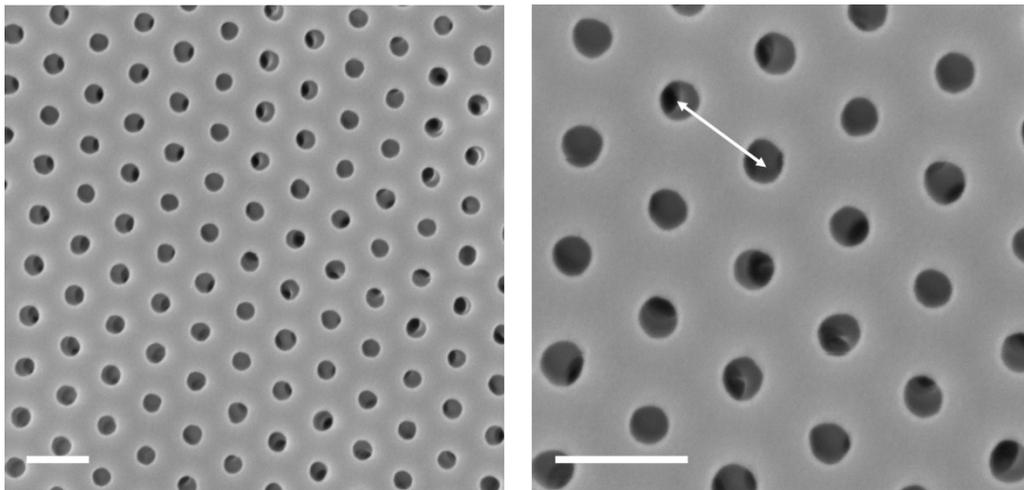
**Figure S1.** SEM images of the surface of the inverse opal structure made with 420 nm beads. The scale bars are 500 nm. The nanopores are stacked in a hexagonally arrangement highly ordered on a large-scale. The arrow indicates the center-to-center distance between two neighboring air cavities, which represents the lattice constant and it is equal to 420nm (the same of the diameter of PS spheres used).
