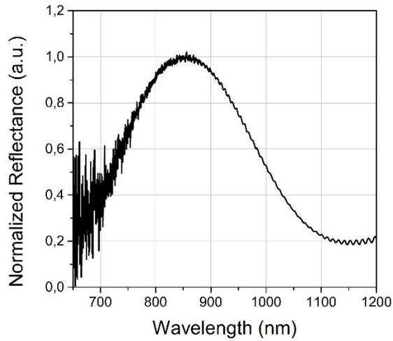
**Figure S2.** Reflectance spectrum of a simple 3 layer silk inverse opal obtained by replica of an opal template made with 420nm beads without a defect layer.
