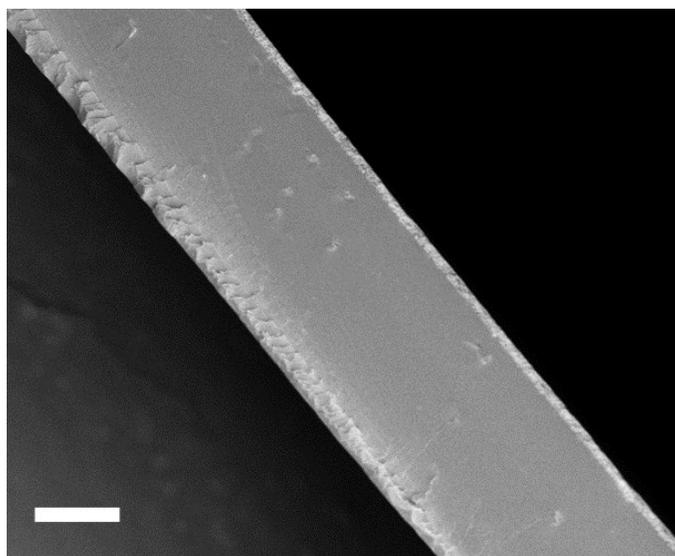
**Figure S5.** Cross-section SEM images of the free-standing SiO<sub>2</sub> film (the scale bar is 20 μm).
