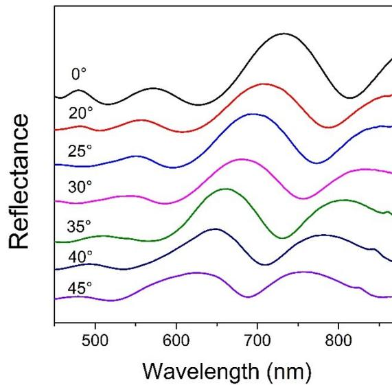
**Figure S3.** Experimental reflectance spectra of a SIO structure including a defect-layer measured from  $\theta = 0^\circ$  (top) to  $\theta = 45^\circ$  (bottom) in steps of  $5^\circ$  (angles between  $5^\circ$  and  $15^\circ$  could not be reported due to limitations of the experimental setup). The shift of the reflection-dip wavelength matches with what could be calculated by using the Bragg-Snell law.
