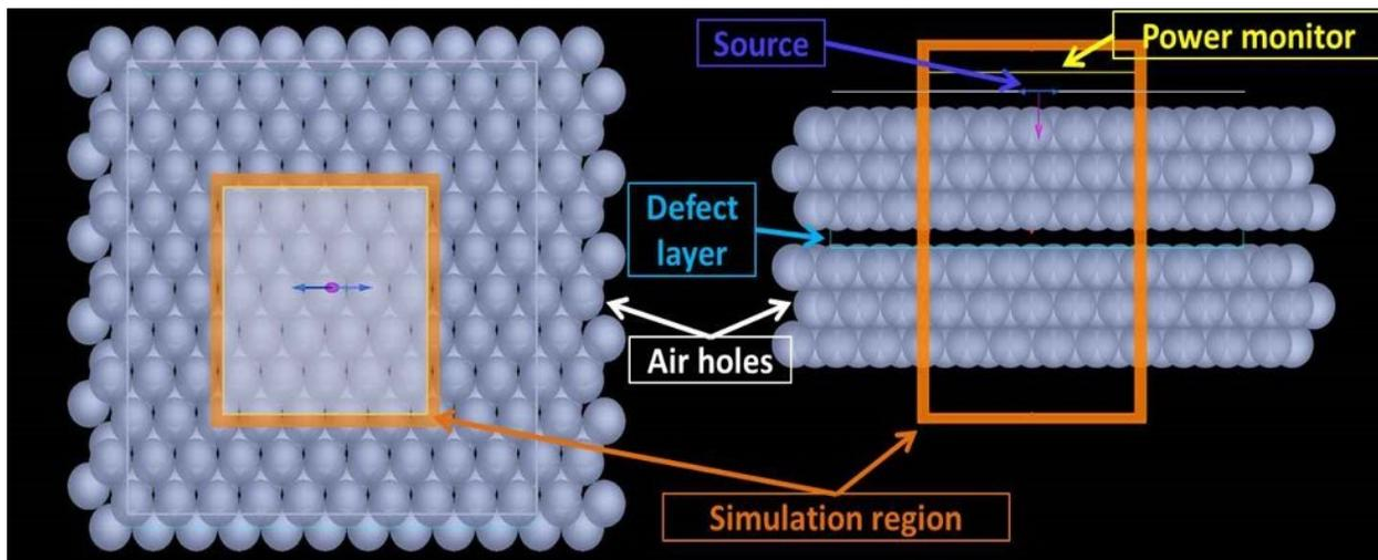
**Figure S4.** Schematic illustration of the structure used for the FDTD simulations. A plane-wave source was placed in close proximity of the opal surface (@ 135-nm distance) and reflectance was measured 235 nm away from the opal surface.
