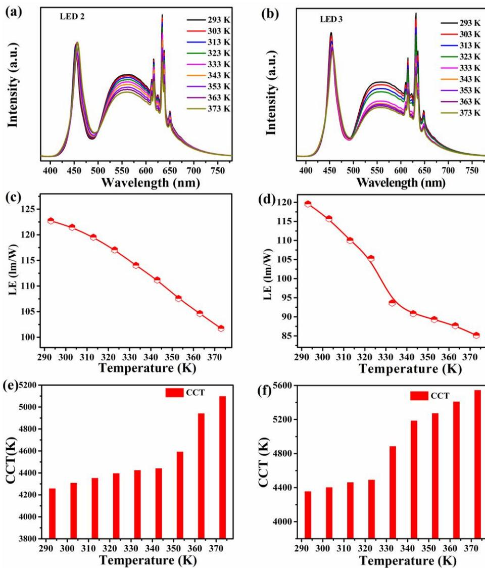
**Fig. S7** Temperature-dependent photoelectric properties of warm LED 2 and LED 3 with temperature varying from 293 K to 373 K: EL spectra (a), LE (c) and CCT (e) for LED 2; EL spectra (b), LE (d) and CCT (f) for LED 3.
