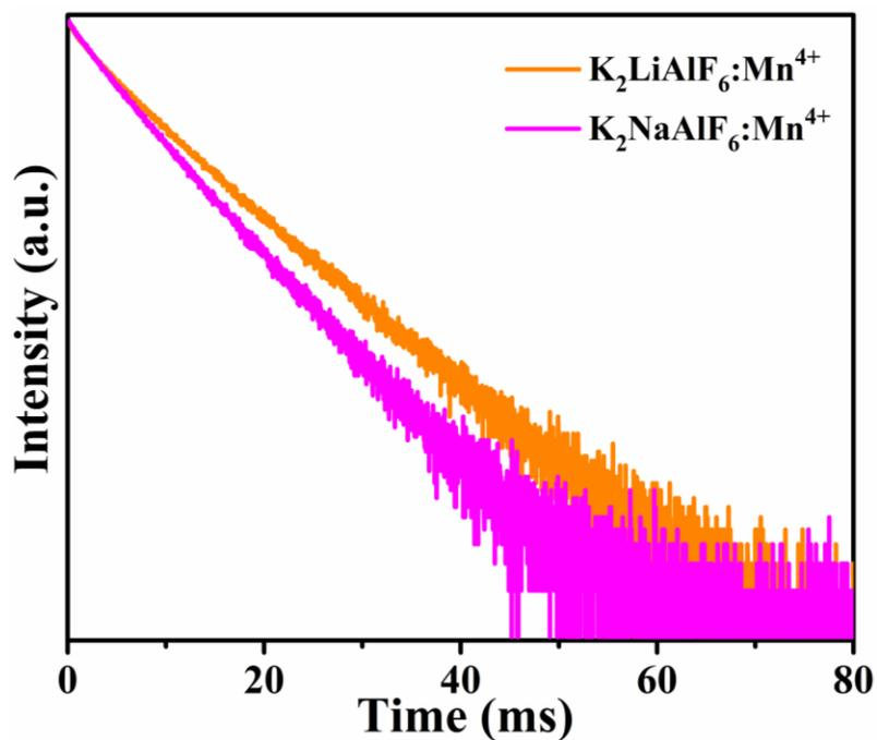
**Fig. S5** PL decay curves of  $\text{K}_2\text{BAlF}_6:\text{Mn}^{4+}$  ( $B = \text{Li}, \text{Na}$ ) at room temperature.
