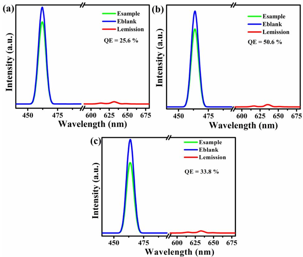
**Fig. S3** Excitation line of blank ( $\text{BaSO}_4$ ) (*Eblank*) and excitation (*Esample*) and emission (*Lemission*) spectra of  $\text{Rb}_2\text{KAlF}_6:\text{Mn}^{2+}$  (a),  $\text{Cs}_2\text{KAlF}_6:\text{Mn}^{2+}$  (b), and  $\text{Cs}_2\text{RbAlF}_6:\text{Mn}^{2+}$  (c). The quantum efficiency (QE) can be calculated as follows:
