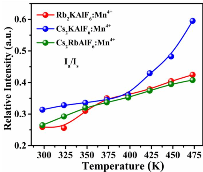
**Fig. S4** The ratio of  $I_a/I_s$  for  $A_2BAlF_6:\text{Mn}^{4+}$  ( $A = \text{Rb}, \text{Cs}; B = \text{K}, \text{Rb}$ ) as a function of temperature at 298 - 473 K.
