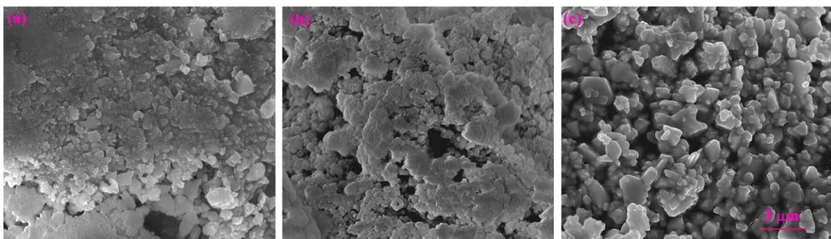
**Fig. S1** SEM images of  $Rb_2KAlF_6:Mn^{4+}$  (a),  $Cs_2KAlF_6:Mn^{4+}$  (b), and  $Cs_2RbAlF_6:Mn^{4+}$  (c) synthesized via same reaction environment. The scale bar in the SEM images is fixed at 3  $\mu m$ .
