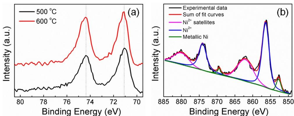
Fig. S4 (a) XPS spectra of Pt 4f in NiO<sub>x</sub>/Pt NWs oxidized at 500 °C and 600 °C. (b)
