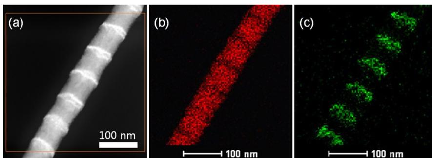
Fig. S2 (a) HAADF-STEM image of Ni/Pt NW and elemental maps of (a) Ni and (b) Pt.
