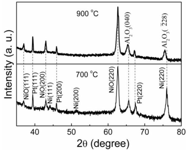
Fig. S1 XRD patterns of the multilayered NiO<sub>x</sub>/Pt NW arrays oxidized at 700 °C and 900 °C.
