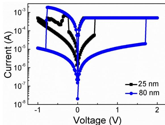
Fig. S6  $I$ - $V$  curves of multilayered NiO<sub>x</sub>/Pt NW devices with different NiO<sub>x</sub> thicknesses.
