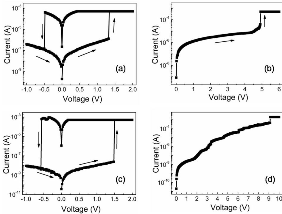
Fig. S5  $I$ - $V$  curves of multilayered  $\text{NiO}_x/\text{Pt}$  NW devices oxidized at 700 °C (a) and 900 °C (c); (b) and (d) are the corresponding electroforming processes.
