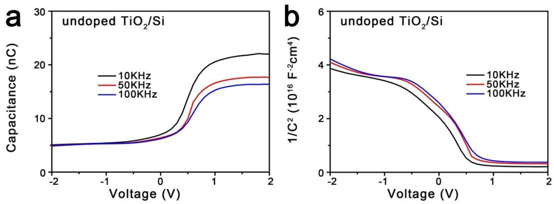
**Figure S3.** The capacitance-voltage characteristic (a) and  $1/C^2$  versus  $V$  plots (b) of the undoped  $\text{TiO}_2/\text{Si}$  heterojunctions, measured in the dark at the frequencies of 10 kHz, 50 kHz and 100 kHz at room temperature.
