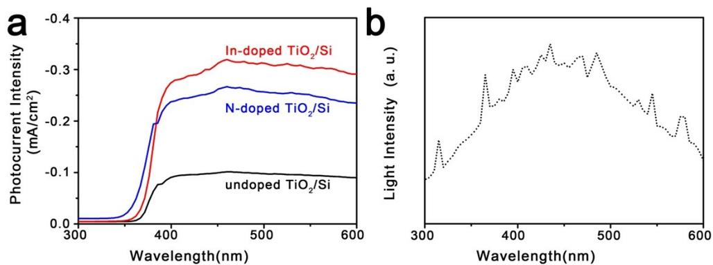
**Figure S9.** (a) The photocurrent spectra of the undoped TiO<sub>2</sub>/Si, In-doped TiO<sub>2</sub>/Si and N-doped TiO<sub>2</sub>/Si heterojunctions with an applied reverse bias of -2 V. (b) Light intensity distribution along the wavelength of Xenon lamp.
