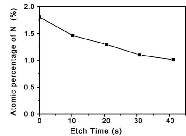
**Figure S7.** The relationship between the percentage of N atoms and the etching time.
