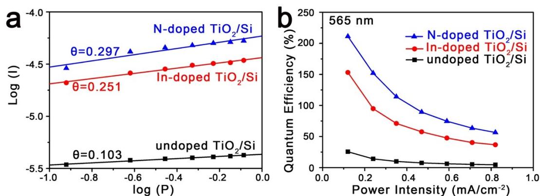
**Figure S11.** The logarithmic form of the photocurrent vs light power intensity (a) and the quantum efficiency (b) at -2 V for the undoped TiO<sub>2</sub>/Si, In-doped TiO<sub>2</sub>/Si and N-doped TiO<sub>2</sub>/Si heterojunctions under 565 nm light illumination, respectively.
