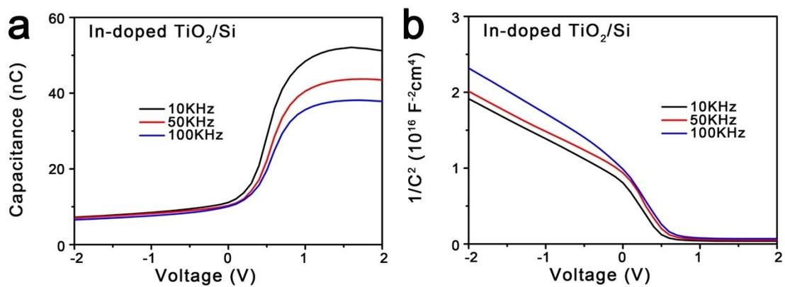
**Figure S4.** The capacitance-voltage characteristic (a) and  $1/C^2$  versus  $V$  plots (b) of the In-doped  $\text{TiO}_2/\text{Si}$  heterojunctions, measured in the dark at the frequencies of 10 kHz, 50 kHz and 100 kHz at room temperature.
