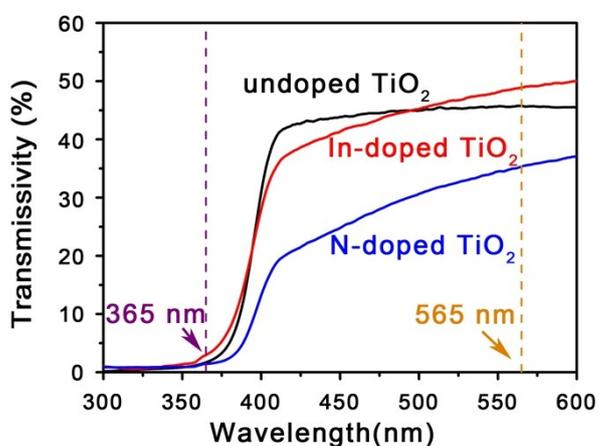
**Figure S10.** The transmittance of the undoped TiO<sub>2</sub>, In-doped TiO<sub>2</sub> and N-doped TiO<sub>2</sub> from 300 nm to 600 nm.
