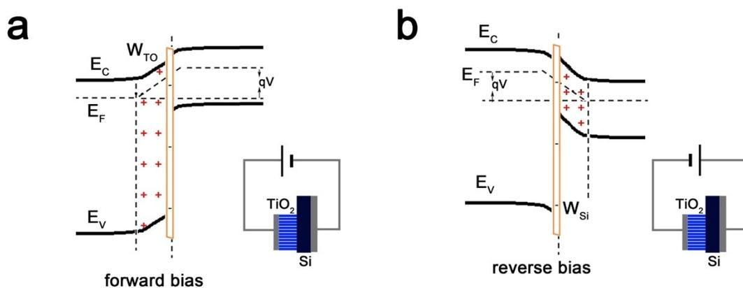
**Figure S2.** Schematic representation of the band energies and internal electrical field of the  $\text{TiO}_2/\text{Si}$  heterojunctions with forward bias (a) and reverse bias (b), respectively.
