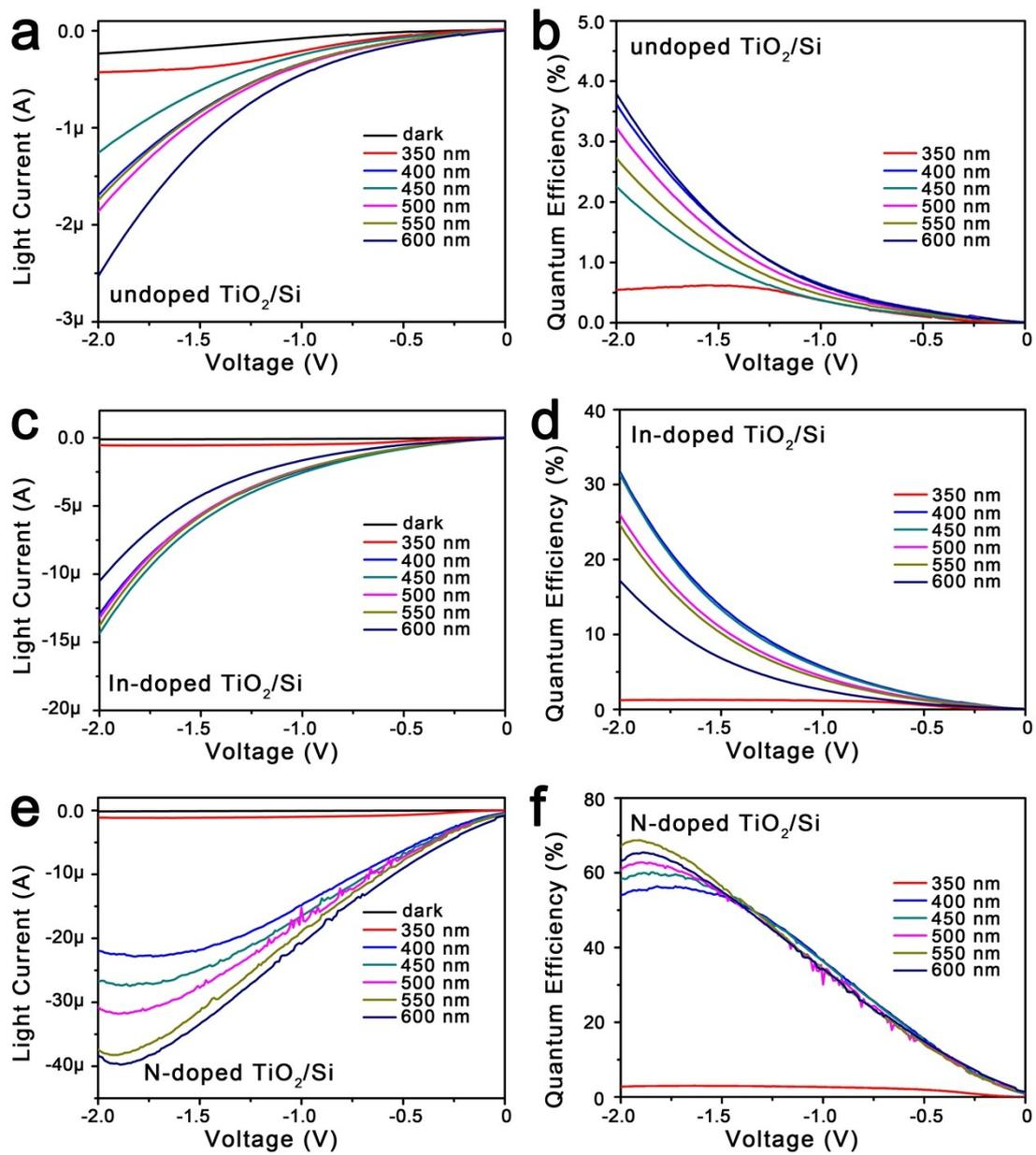
**Figure S8.** The light I-V curves (a, c and e) and the converted quantum efficiency (b, d and f) of the undoped TiO<sub>2</sub>/Si, In-doped TiO<sub>2</sub>/Si and N-doped TiO<sub>2</sub>/Si heterojunctions at a reverse bias under dark, 350 nm, 400 nm, 450 nm, 500 nm, 550 nm and 600 nm, respectively. Here, the light intensity is 0.5 mW/cm<sup>2</sup>.
