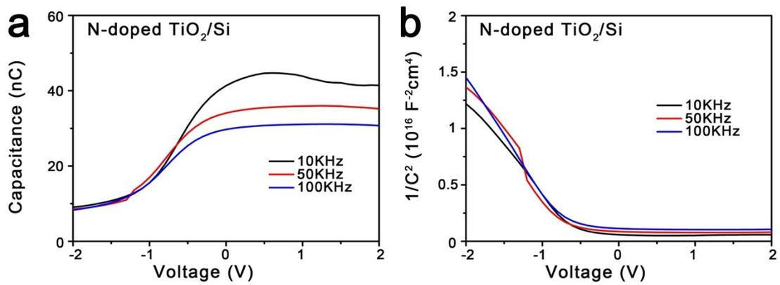
**Figure S5.** The capacitance-voltage characteristic (a) and  $1/C^2$  versus  $V$  plots (b) of the N-doped  $\text{TiO}_2/\text{Si}$  heterojunctions, measured in the dark at the frequencies of 10 kHz, 50 kHz and 100 kHz at room temperature.
