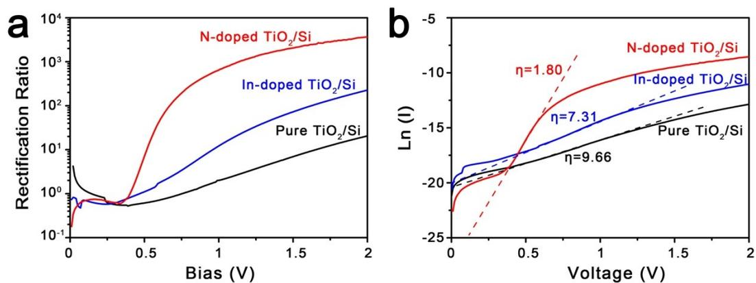
**Figure S1.** (a) The rectification ratios of the undoped  $\text{TiO}_2/\text{Si}$ , In-doped  $\text{TiO}_2/\text{Si}$  and N-doped  $\text{TiO}_2/\text{Si}$  heterojunctions with the bias of 0 V to 2 V. (b)  $\ln(I)$ - $V$  characteristics of those heterojunctions with forward voltage from 0 V to 2 V.
