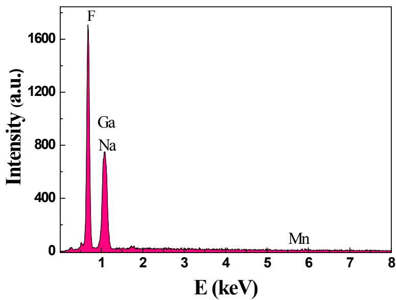
**Figure S4** Energy dispersive spectrum (EDS) of red phosphor  $\text{Li}_3\text{Na}_3\text{Ga}_2\text{F}_{12}:\text{Mn}^{4+}$ .
