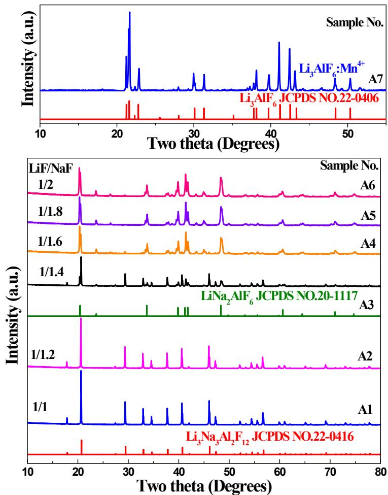
**Figure S2** XRD patterns of samples prepared from LiF, NaF, and  $\text{AlF}_3 \cdot 3\text{H}_2\text{O}$  according to the molecular ratios list in Table S2.
