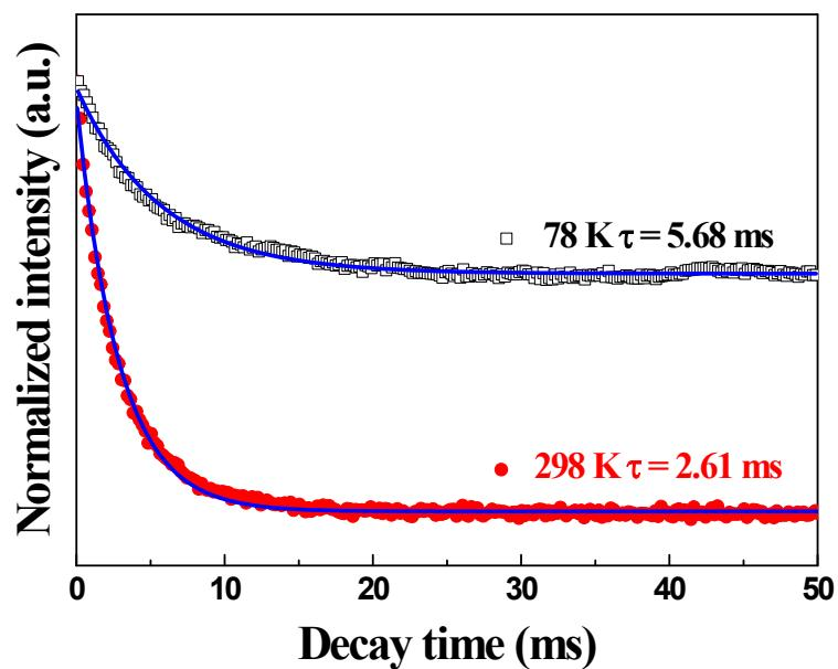
**Figure S5** Decay curves of 629 nm emission of red phosphor  $\text{Li}_3\text{Na}_3\text{Ga}_2\text{F}_{12}:\text{Mn}^{4+}$  excited at 467 nm measured at 78 and 298 K.
