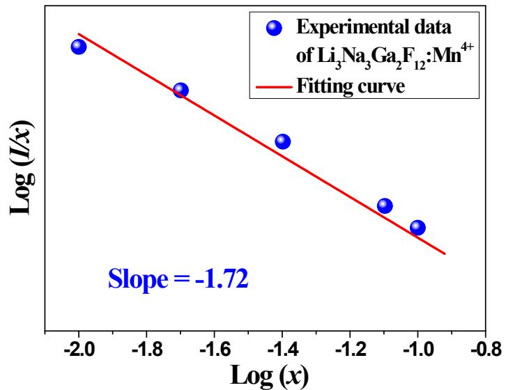
**Figure S6** The relationship between  $\log (x)$  versus  $\log (I/x)$  in the phosphor  $\text{Li}_3\text{Na}_3\text{Ga}_2\text{F}_{12}:\text{Mn}^{4+}$ . (Note:  $x$  is the concentration of  $\text{Mn}^{4+}$ .)
