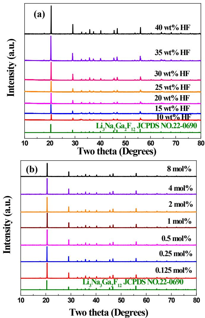
**Figure S3** XRD patterns of samples  $\text{Li}_3\text{Na}_3\text{Ga}_2\text{F}_{12}:\text{Mn}^{4+}$  prepared with various concentrations of (a) HF and (b)  $\text{K}_2\text{MnF}_6$  (mol % of  $\text{Li}_3\text{Na}_3\text{Ga}_2\text{F}_{12}$ ).
