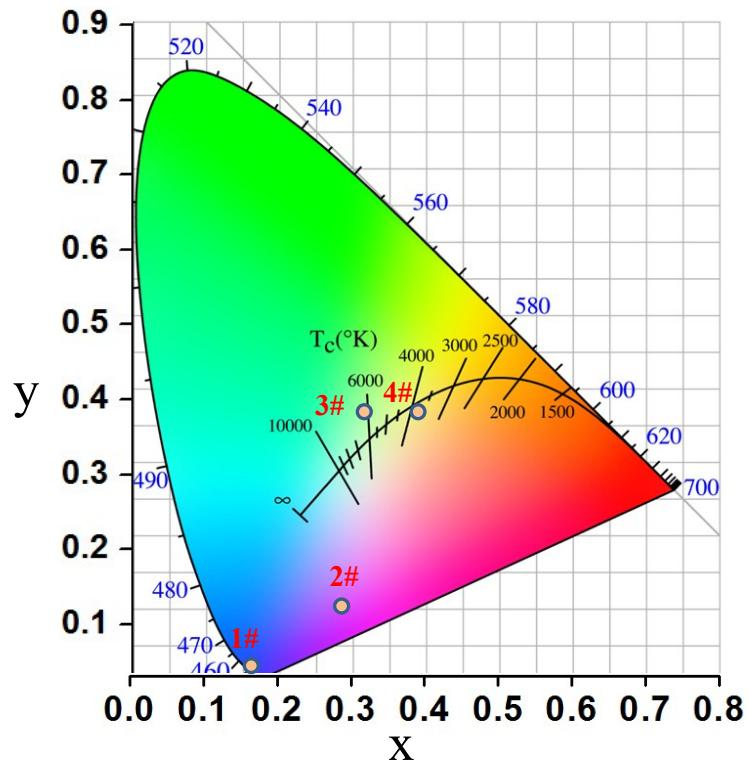
**Figure S8.** CIE chromaticity coordinates, correlated color temperature (CCT) and color rendering index (CRI ) of the as- fabricated LEDs as shown in Fig. 7.
