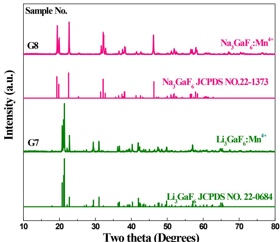
**Figure S1** XRD patterns of samples prepared from LiF, NaF, and  $\text{Ga}_2\text{O}_3$  in HF solution according to the molecular ratios list in Table S1.
