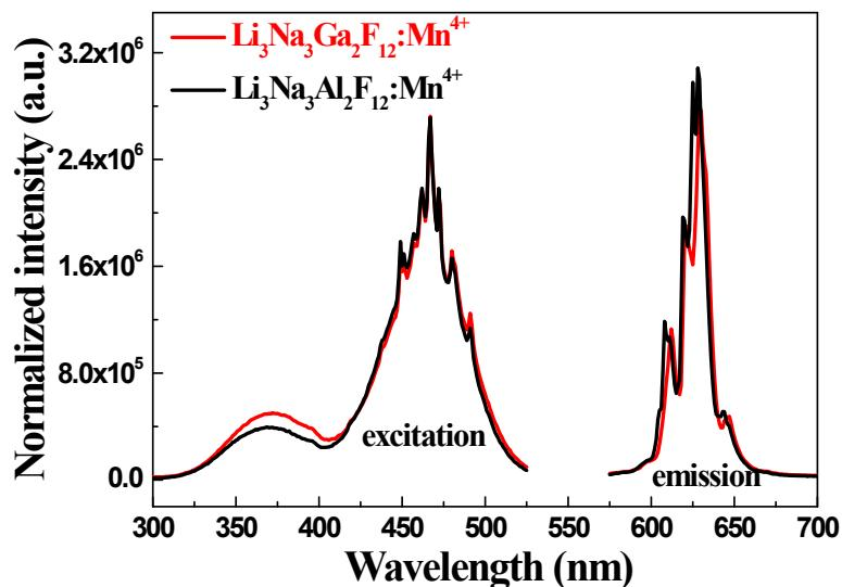
**Figure S7** Excitation (monitored at 629 nm) and emission spectra (excited at 467 nm) of red phosphors  $\text{Li}_3\text{Na}_3\text{Ga}_2\text{F}_{12}:\text{Mn}^{4+}$  and  $\text{Li}_3\text{Na}_3\text{Al}_2\text{F}_{12}:\text{Mn}^{4+}$  with normalized intensities.
