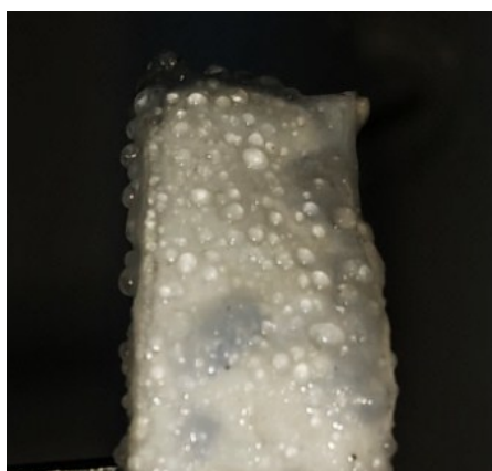
Fig. S2 Optical picture of bubble-like structures on the hydrogel surface formed during the heating process if no PEG was added during the bilayer hydrogel formation.
