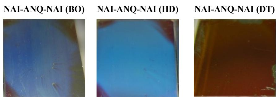
Figure S6. Film quality of **NAI-ANQ-NAI** after spin-coating at 1000 rpm for 60 s
