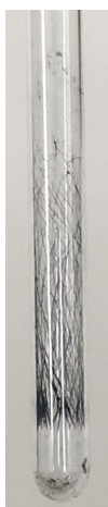
Fig. S4 Crystallization test of DPA-ANT-DPA. The sample is prepared by dropping the chloroform solution into the glass tube and then observed the formation of crystal needles during the solvent drying process.
