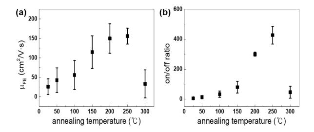
Figure S2 (a)  $\mu_{\text{FE}}$  and on/off ratio of BP FETs vacuum-annealed at different temperatures
