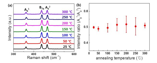
Figure S1 (a) micro-Raman spectra and (b) intensity ratio  $(A_g^{1/}A_g^{2})$  of BP vacuumannealed at different temperatures
