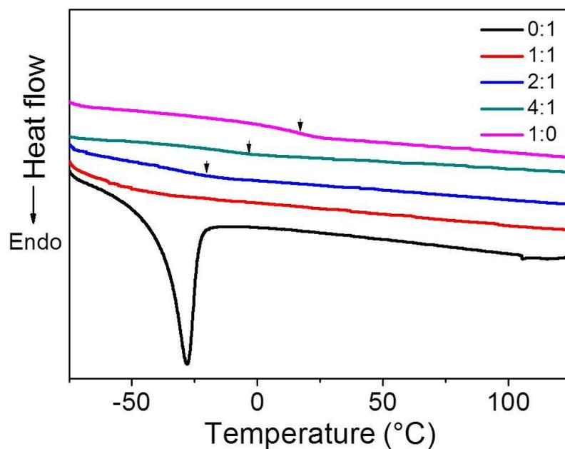
Figure S5. DSC curves of P(BMA-co-LMA)/mMWCNT composites with different molar ratio of BMA/LMA and 7 wt% of mMWCNT content.
