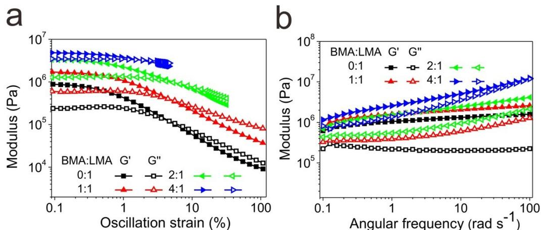
Figure S9. Rheology measurements of the composite containing 10 wt% mMWCNT. (a) Dynamic oscillation strain dependence of storage ( $G'$ , filled symbols) and loss ( $G''$ , open symbols) modulus at  $1 \text{ rad s}^{-1}$  and (b) frequency dependence of  $G'$  and  $G''$  at a strain of 0.5%.
