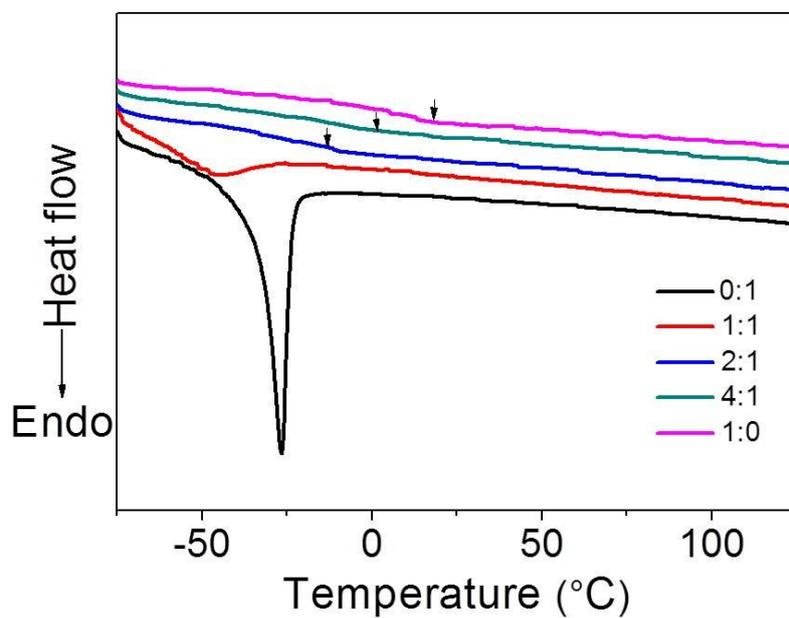
Figure S6. DSC curves of P(BMA-co-LMA)/mMWCNT composites with different molar ratio of BMA/LMA and 10 wt% of mMWCNT content.
