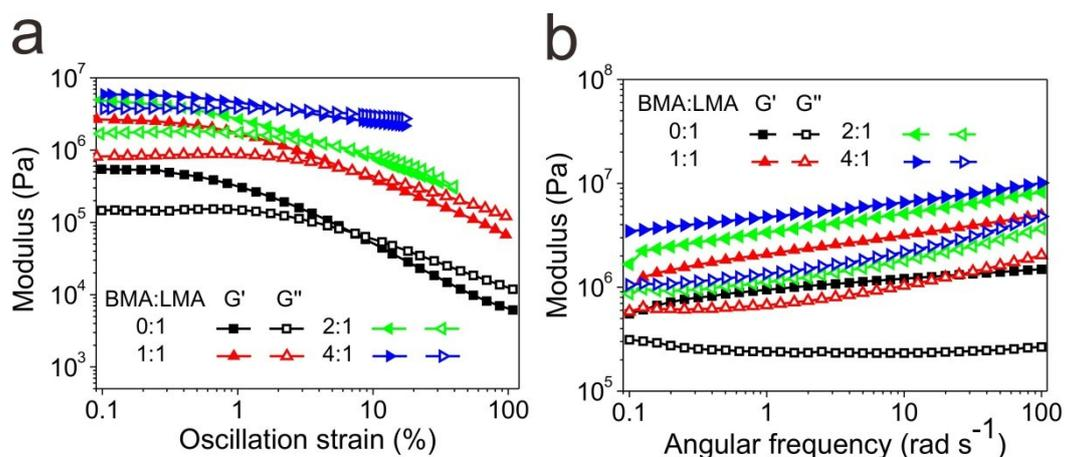
Figure S10. Rheology measurements of the composite containing 13 wt% mMWCNT. (a) Dynamic oscillation strain dependence of storage ( $G'$ , filled symbols) and loss ( $G''$ , open symbols) modulus at  $1 \text{ rad s}^{-1}$  and (b) frequency dependence of  $G'$  and  $G''$  at a strain of 0.5%.
