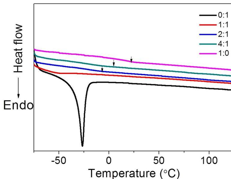
Figure S7. DSC curves of P(BMA-co-LMA)/mMWCNT composites with different molar ratio of BMA/LMA and 13 wt% of mMWCNT content.
