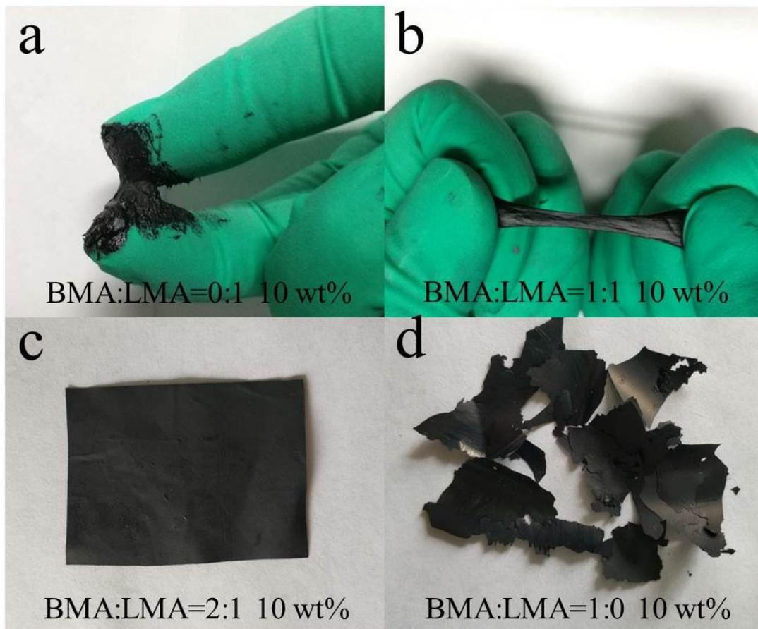
Figure S4. Photograph of P(BMA-co-LMA)/mMWCNT composites with different molar ratio of BMA/LMA and the content of mMWCNT remained at 10 wt%.
