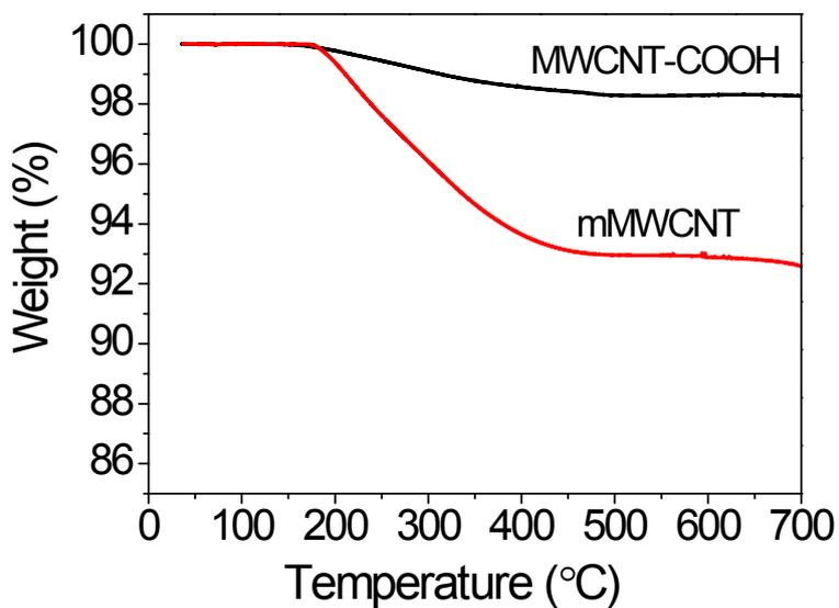
Figure S3. TGA curves of undecylenyl alcohol grafted multiwalled carbon nanotube (mMWCNT) and original acidified MWCNT.
