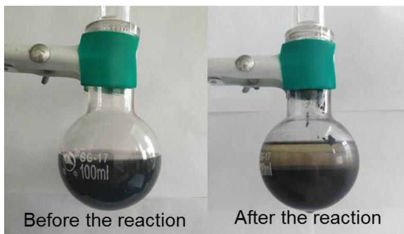
Figure S1. Photograph of the solution before (left) and after (right) multiwalled carbon nanotube reacted with undecylenyl alcohol.
