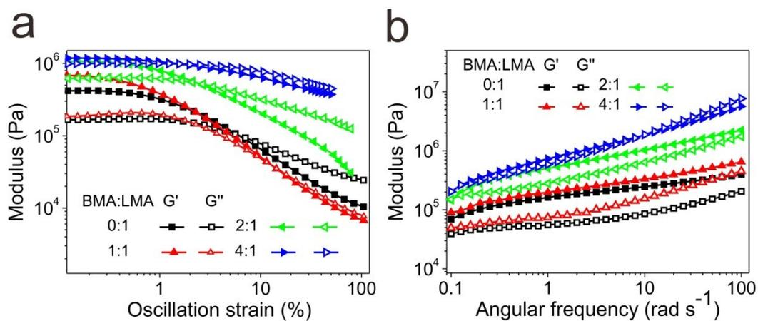
Figure S8. Rheology measurements of the composite containing 7 wt% mMWCNT. (a) Dynamic oscillation strain dependence of storage ( $G'$ , filled symbols) and loss ( $G''$ , open symbols) modulus at  $1 \text{ rad s}^{-1}$  and (b) frequency dependence of  $G'$  and  $G''$  at a strain of 0.5%.
