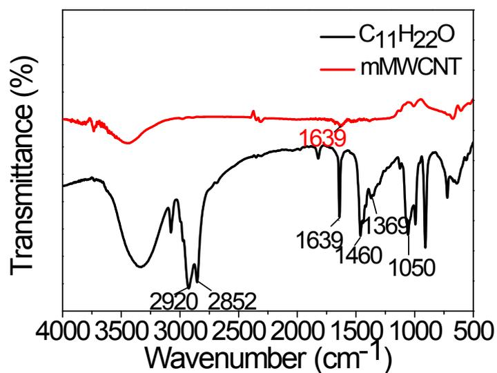
Figure S2. FTIR of undecylenyl alcohol and undecylenyl alcohol modified multiwalled carbon nanotube.
