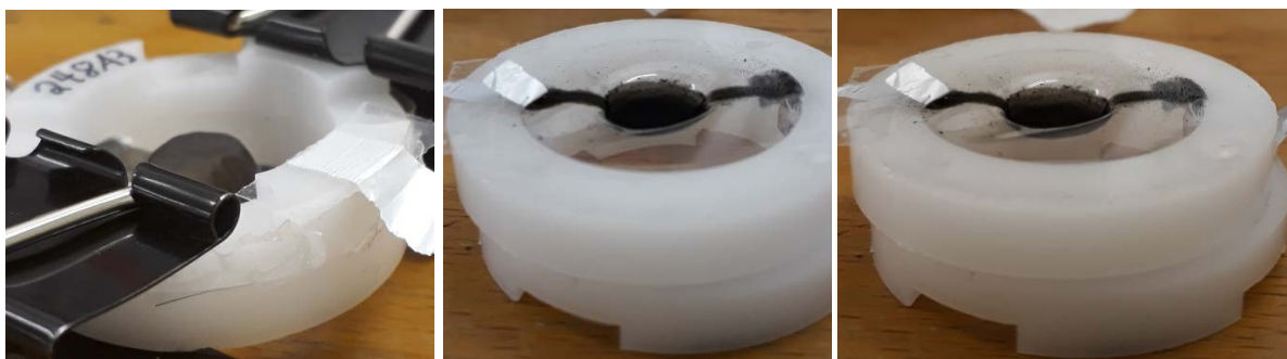
Figure S62. Photos showing that the actuator inflates in both directions.
