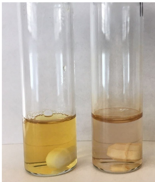
Fig. S6. Photograph showing a comparison of two different reaction solutions: (left) a standard synthesis and (right) a synthesis with the introduction of NaCl instead of CTAC. When replacing CTAC with NaCl, severe aggregations were observed in the reaction solution.
